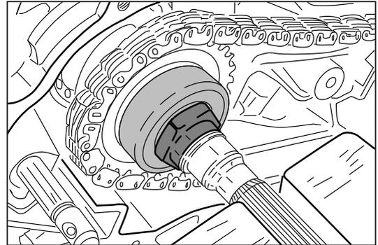
18. Insert the speedometer drive gear to the transfer output rear shaft.
