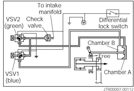
2. When center differential lock switch is turned on.
