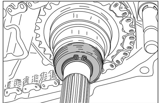
20. Install new "O" ring to the transfer fork shaft.
