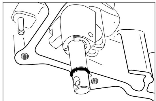
21. Apply the liquid gasket interposed, assemble the transfer case and transfer case No. 2 by tapping it evenly and lightly at the rib sections (A), (B) and (C) by means of a plastic hammer or the like.
