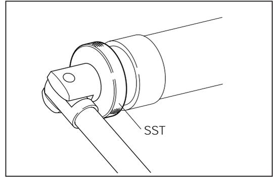
6. Remove the rack cover tube installed to the power steering rack sub-assembly.
