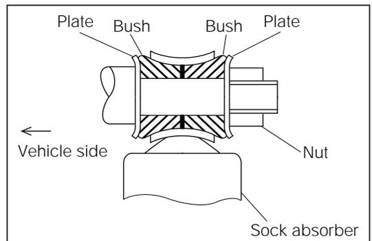
2. Install the shock absorber to the shock absorber attaching stud bolt.
