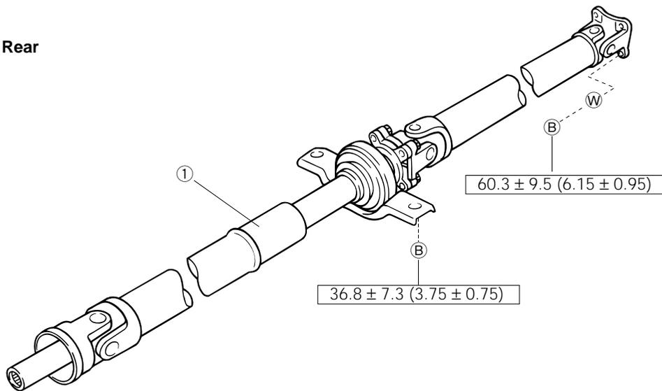
① Propeller shaft assembly
