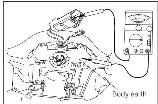
2. Checking procedure of air bag at the passenger's seat side
