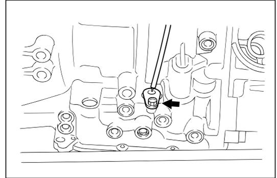
32. Removal of 2nd brake piston assembly
