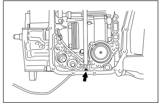
30. Remove the solenoid wire assembly attaching bolt.
