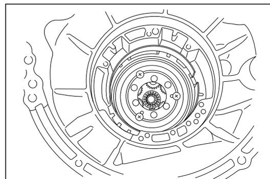
14. Assembly of forward clutch hub and 2nd brake drum
