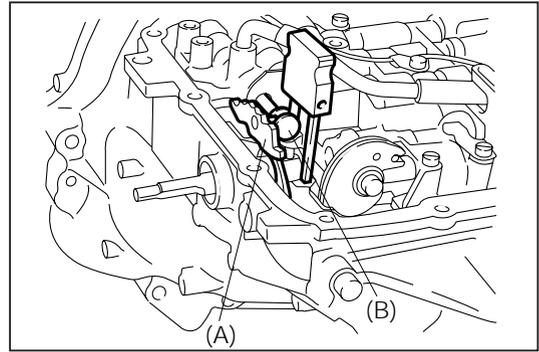
(4) Tighten the bolts of the valve body assembly.
