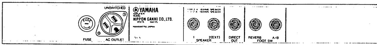
The illustration shows the U.S. and CANADIAN models. Other models are equipped with voltage selectors instead of AC outlets. So be sure to check for desired voltage.
