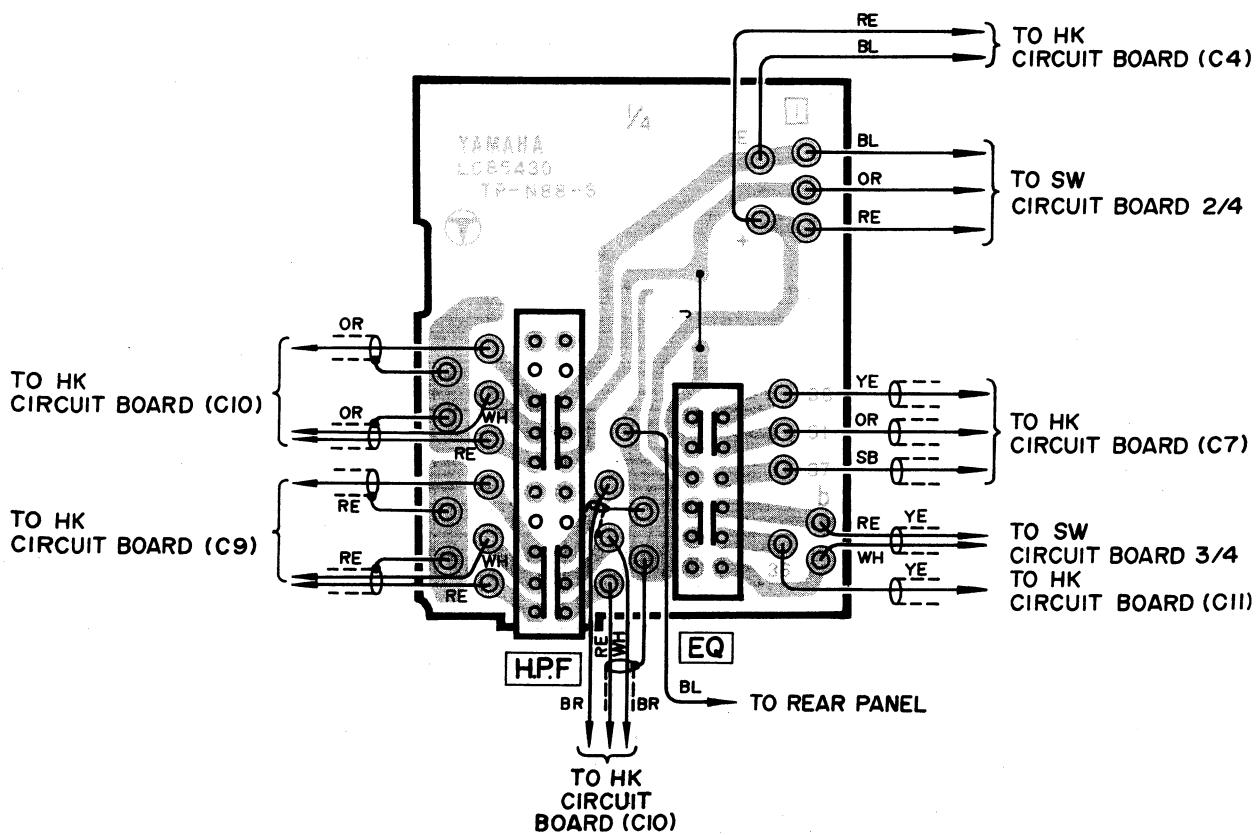
• DC CIRCUIT BOARD 1/3 NA80591 (Parts Side)
