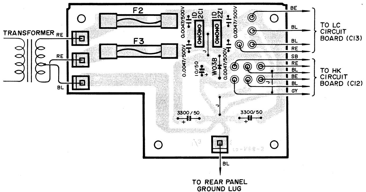
• WIRING CIRCUIT BOARD 2/3, 3/3 NA80591 (Pattern Side)
