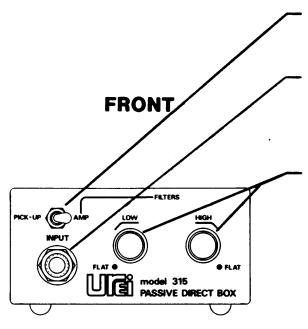
**INPUT SWITCH.** Selects correct input signal conditioning.
