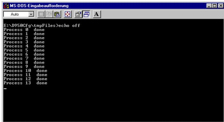
First all channels and then all the summing busses are allocated to the required DSP board processors. Then the final core file is assembled out of individual components:
