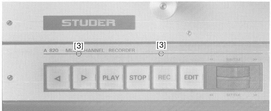
Fig. 51 Drucktastenaggregat
