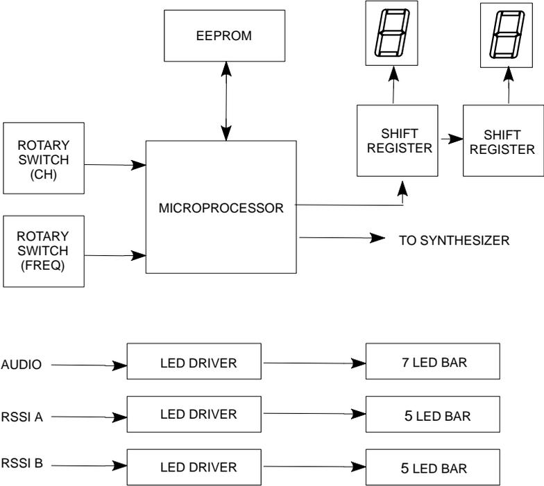
Figure 4. UC4 Digital and Display Section Block Diagram
