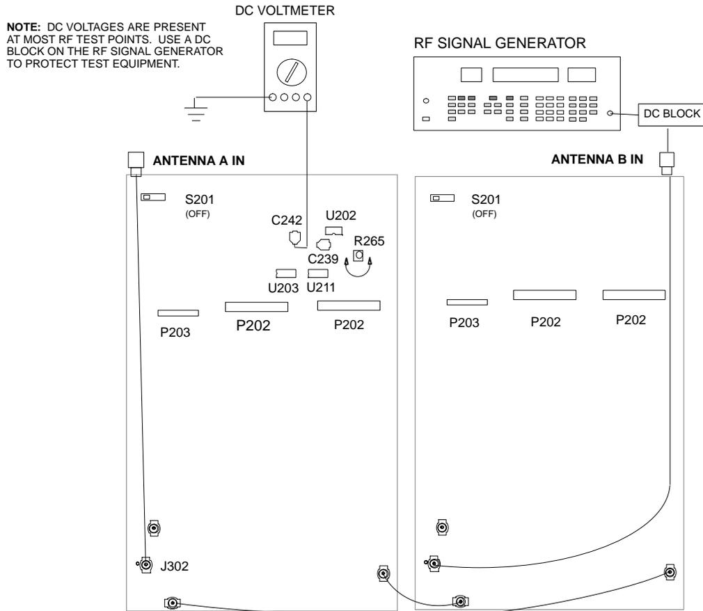
**Figure 14.** Channel B, Noise Setup Connections
