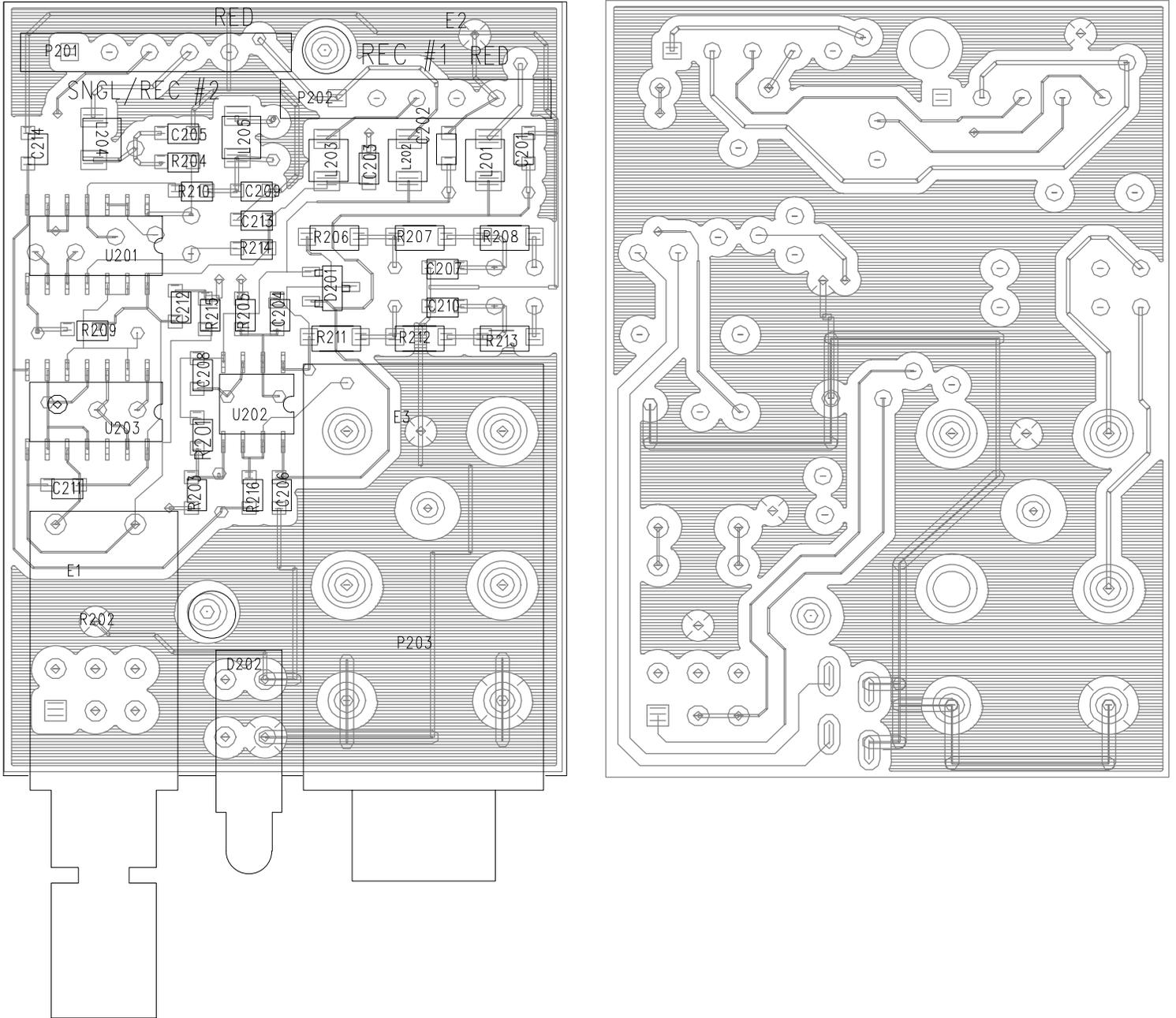
**Figure 19.** Headphone Monitor Printed Circuit Board Legend
