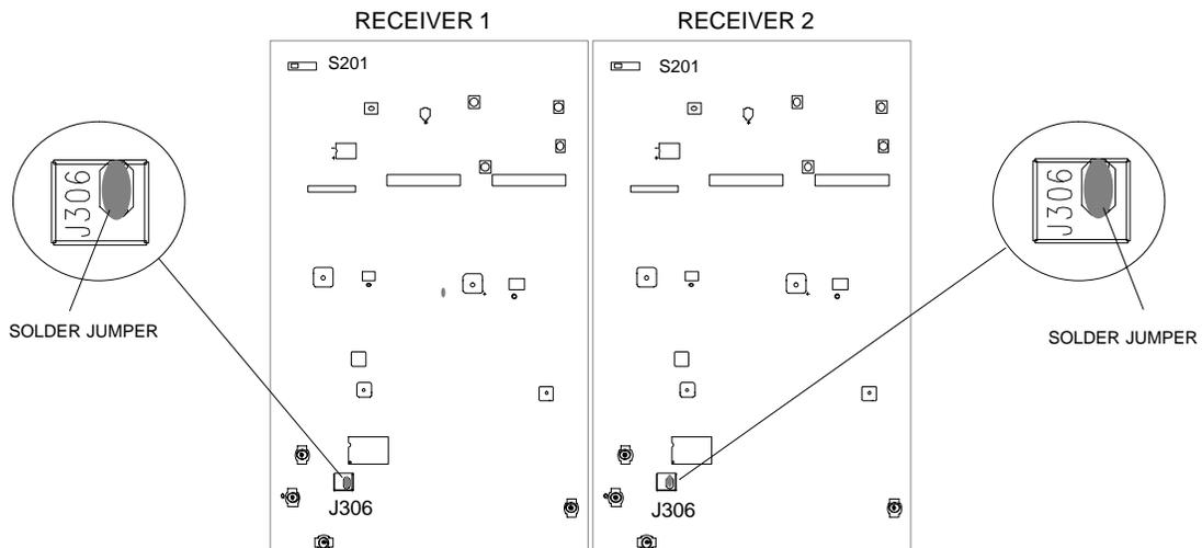
**Figure 4.** U4D Receiver Solder Jumper Locations
