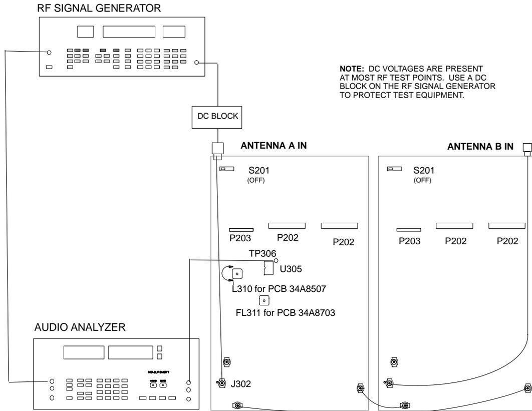
**Figure 7.** FM Detector Quadrature Coil Alignment Connections
