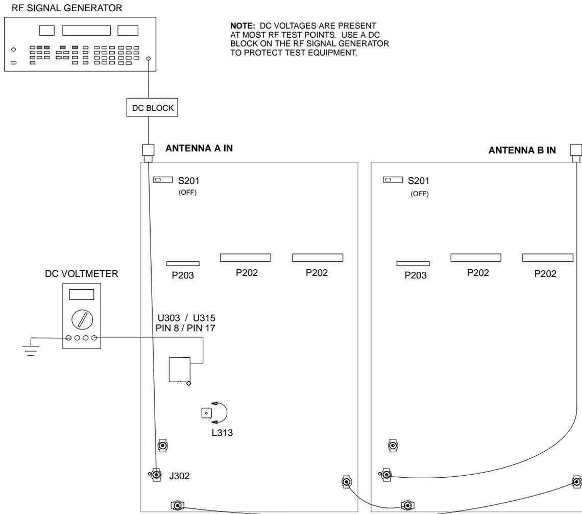
**Figure 8.** Channel A Second Mixer Coil Alignment
