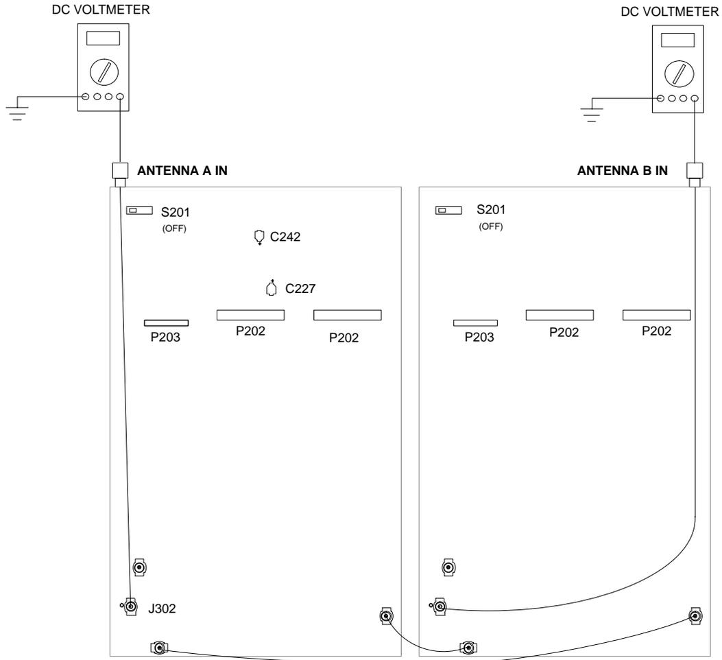
**Figure 5.** Dc Voltage Level Verification
