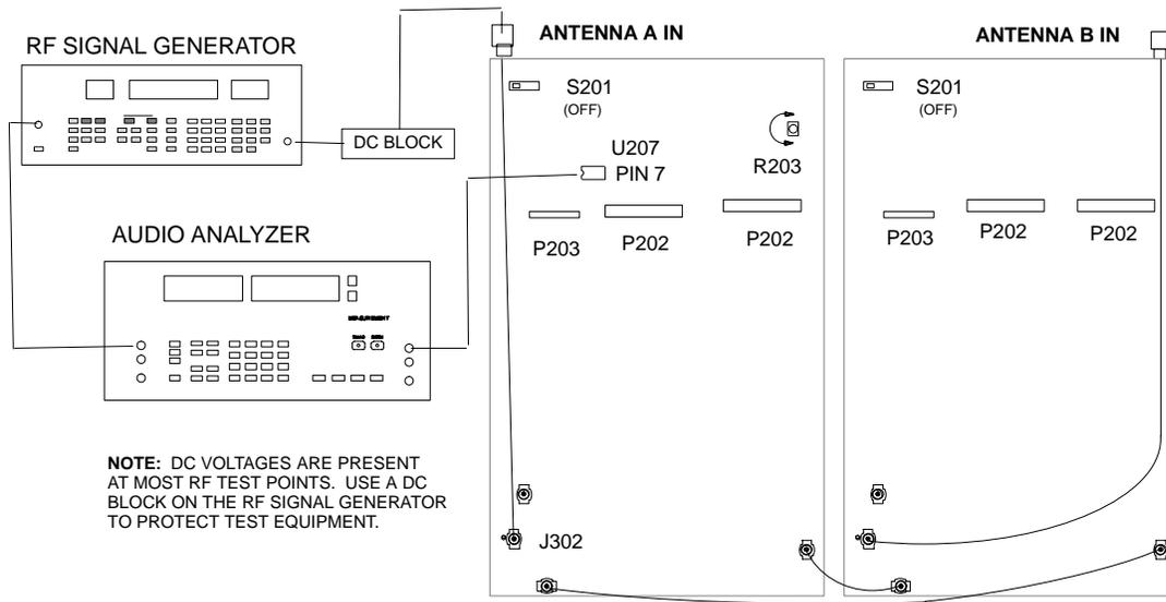
**Figure 16.** Channel A Audio Level Setup Connections
