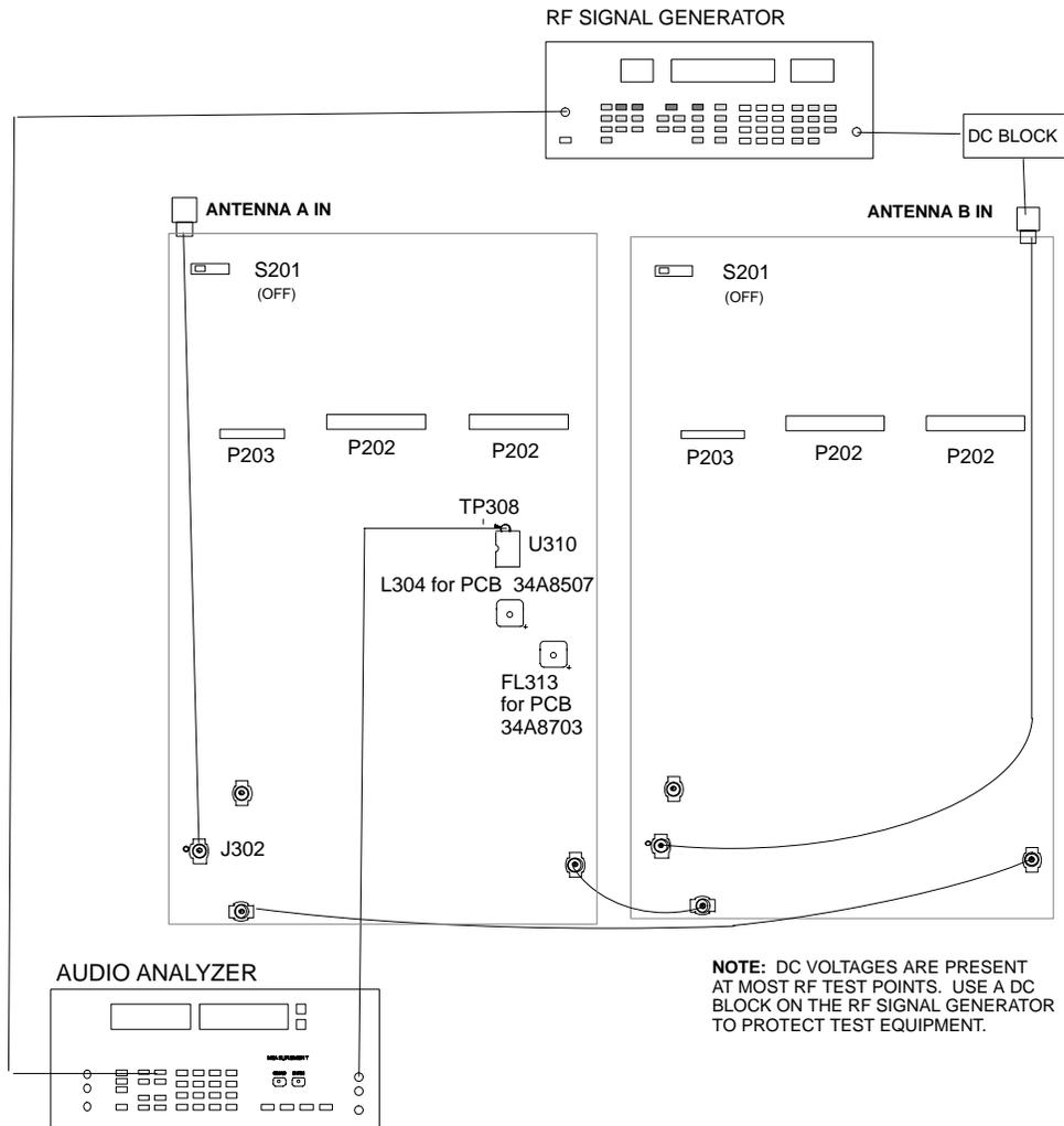
**Figure 11.** Channel B FM Detector Quadrature Coil Alignment
