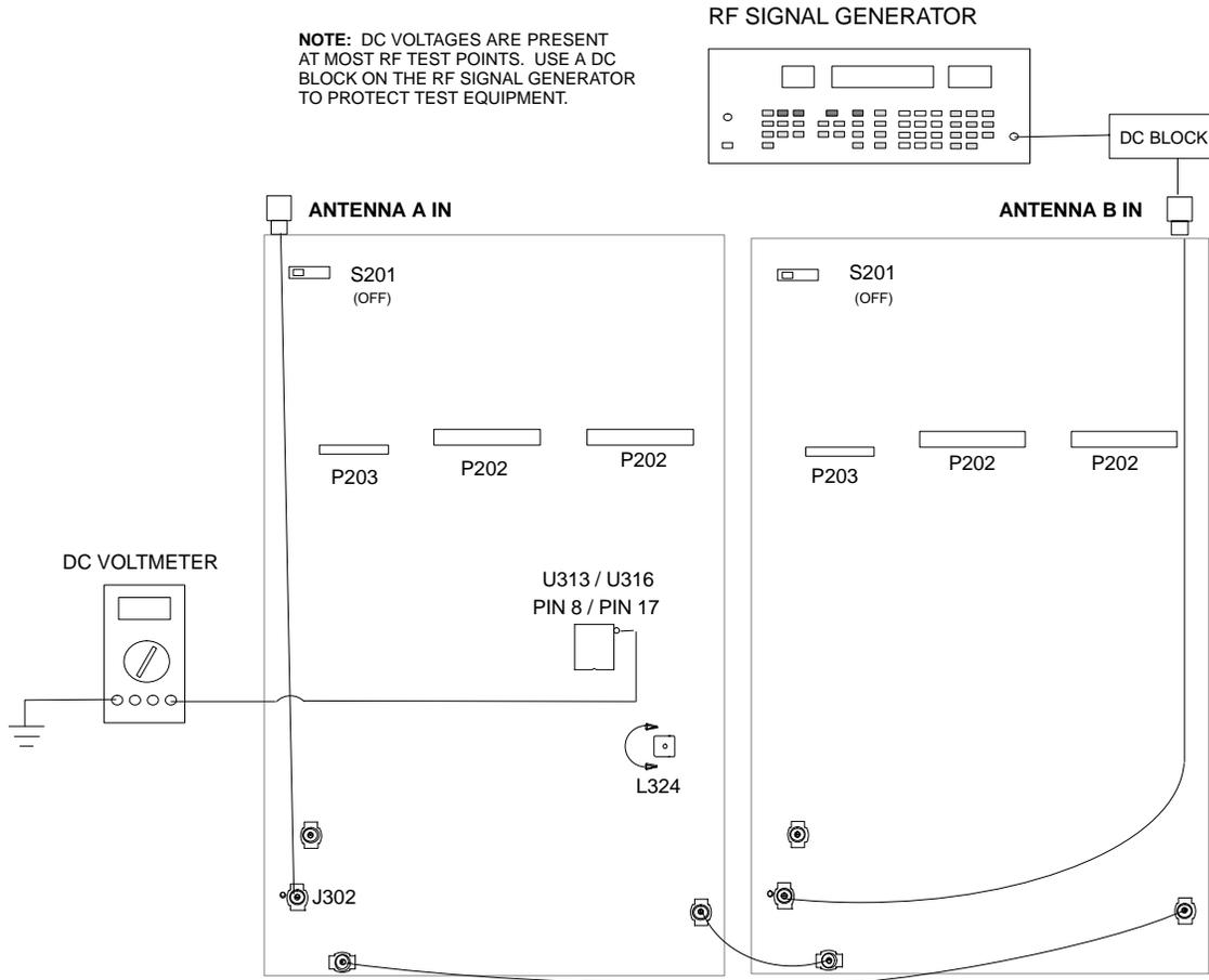
**Figure 12.** Channel B Second Mixer Coil Adjustment Connections
