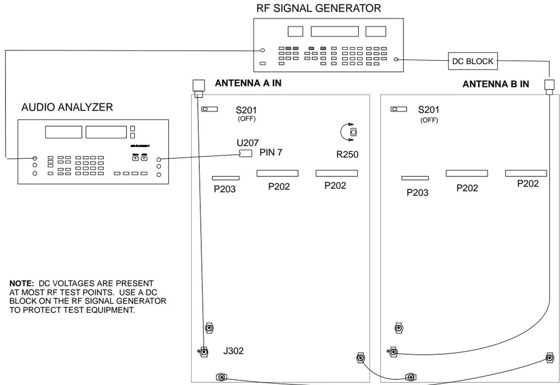
**Figure 15.** Channel B Audio Level Setup Connections
