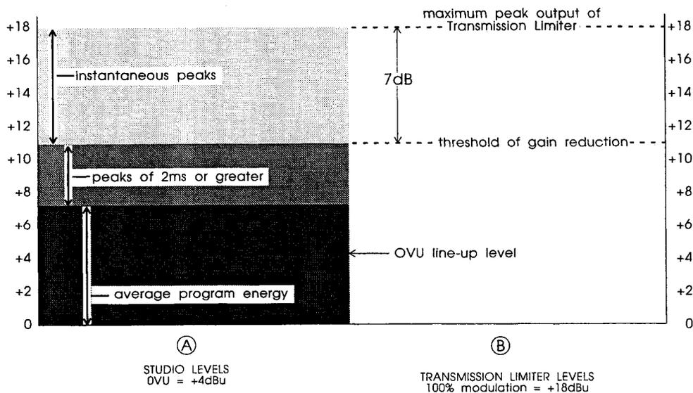
Figure 1-3: Level Calibration — US-style Facilities
