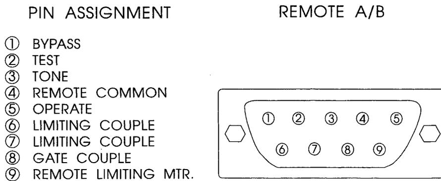
Figure 2-9: Rear Panel Remote Control/Stereo Coupling
