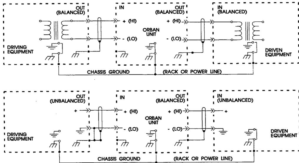
Figure 2-10: Typical Interconnection, Grounding Scheme
