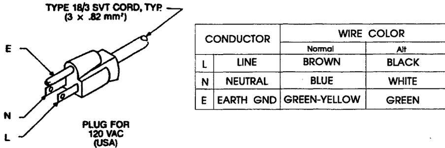
Figure 2-1: Line Cord Wiring Standard
