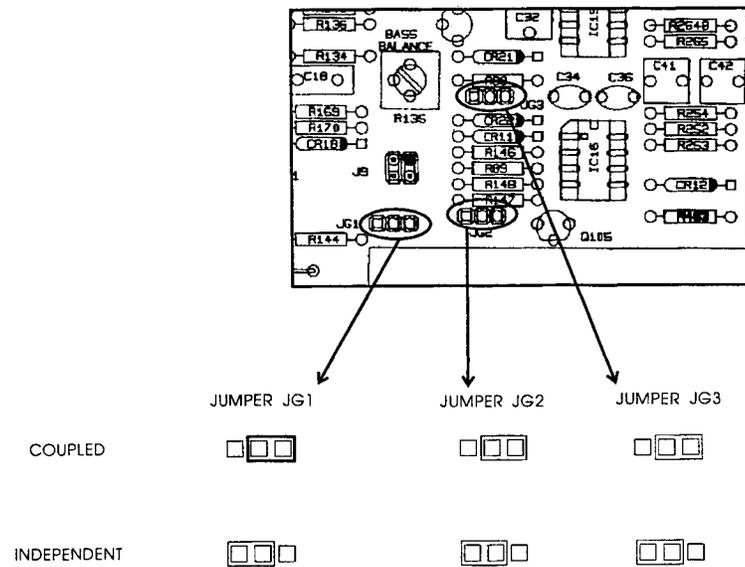
Figure 2-8: Stereo Coupling
