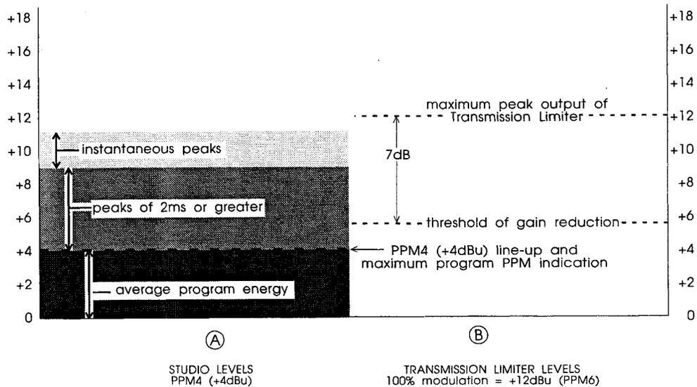
Figure 1-5: Level Calibration — With BBC-Standard PPM
