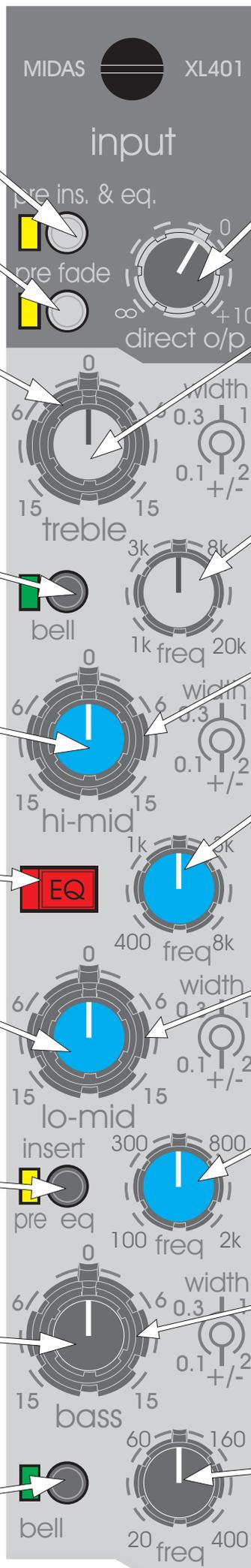
The DIRECT output control gives continuous adjustment of the direct output level from + 10dB to off. The output is derived from the input channel post fader signal.
