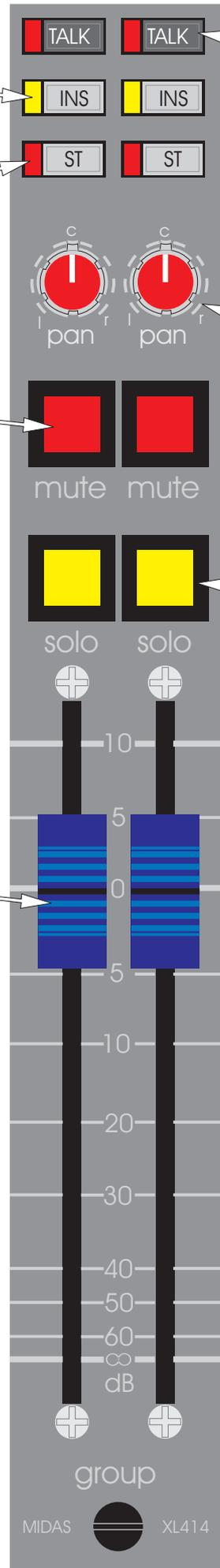
The TALK switches connect the audio sub groups to the COMMS module. When the TALK TO GROUPS switch on the COMMS module is activated it is then able to route its oscillator, pink noise, external input, talk mic or comms mic to the audio sub groups.
