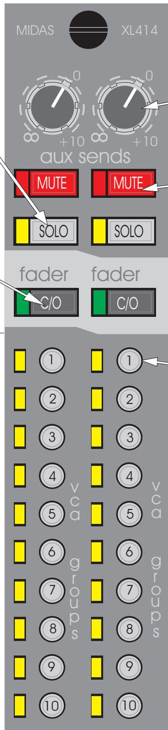
The AUX SEND controls give continuous adjustment of the mono aux bus output levels from + 10dB to off.
