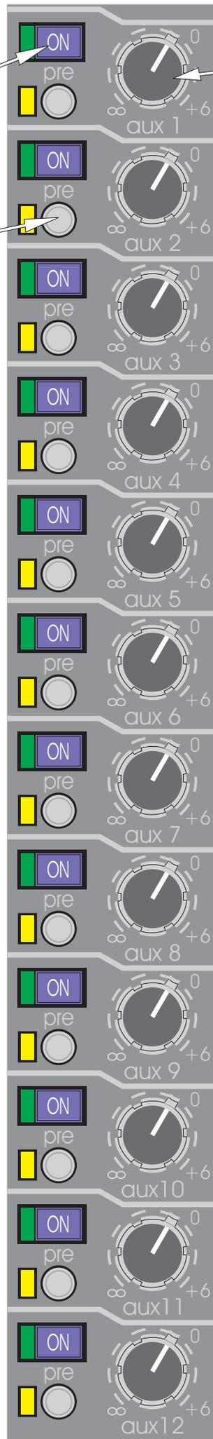
The mono AUX controls ( 1 to 16 ) give continuous adjustment of the level sent from the input channel to the aux busses. The level adjustment is from +6dB to off.
