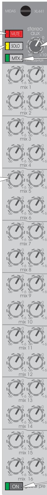
The STEREO AUX MASTER control gives continuous adjustment of the stereo aux output level from + 10dB to off.
