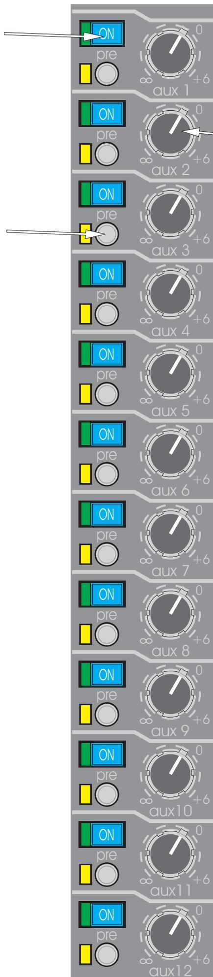
The mono AUX controls (1 to 16) give continuous adjustment of the level sent from the input channel to the aux busses. The signal is a mono sum of the left and right signals and the level adjustment is from +6dB to off.
