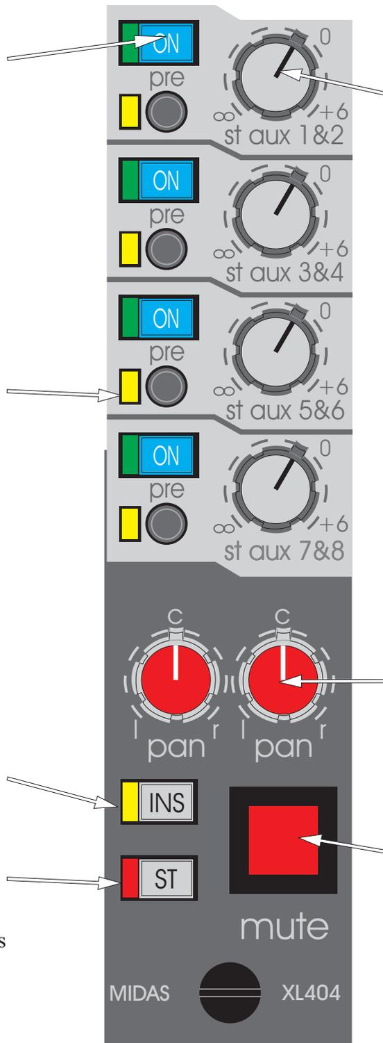
The ST AUX controls (1 to 8) give continuous adjustment of the level sent from the input channel (post pan) to the stereo aux busses. The level adjustment is from +6dB to off.
