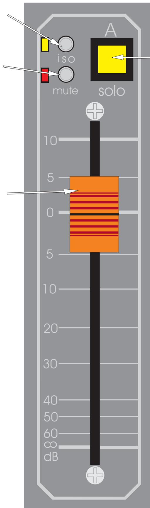
The grand master A and B vca SOLO switches are used to monitor the grand master A and B VCA sub groups by creating a corresponding AUDIO sub groups on the stereo AFL busses. All AUDIO sub groups that are assigned to grand master vca A or B will be summed onto the solo busses when the vca solo is active.
