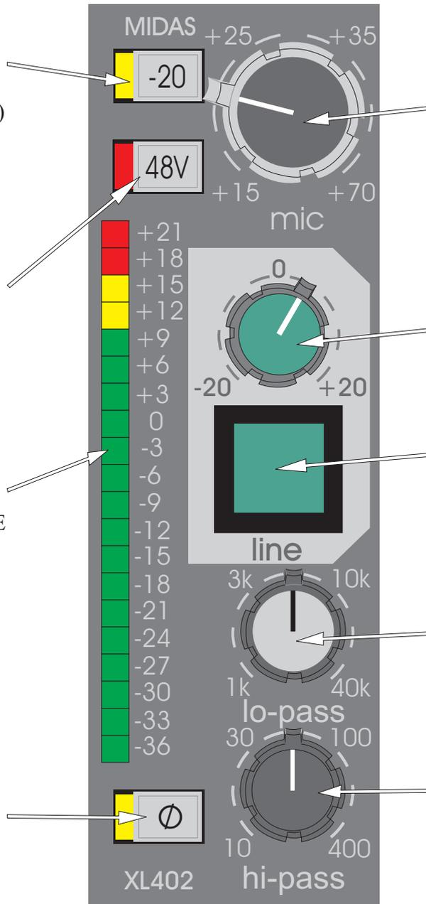
The MIC control gives continuous adjustment of the mic amp gain from + 15dB to + 70dB.
