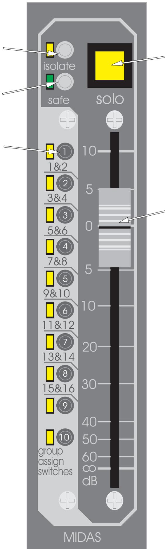
The SOLO switch sends the input channel signal to the PFL mono and AFL stereo busses. If the switch is pressed for a short time it will latch on or off, but, if it is held on for more than 1 second the latching is disabled and when the switch is released the channel solo will turn off.
