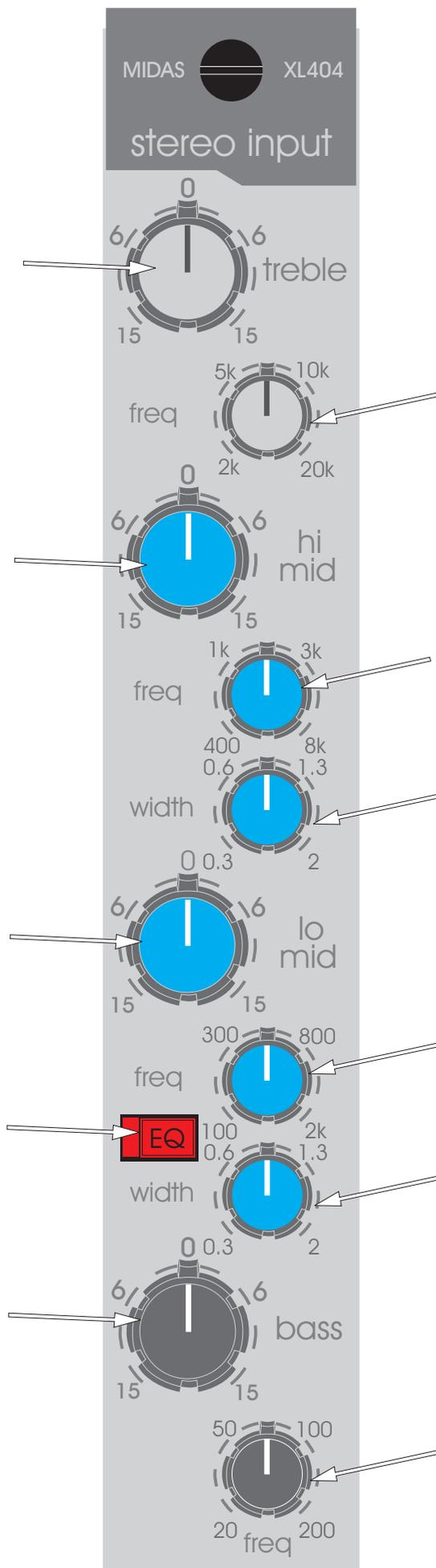
The treble FREQ control gives continuous adjustment of the frequency range that the treble equalisers act on from 2K to 20K.
