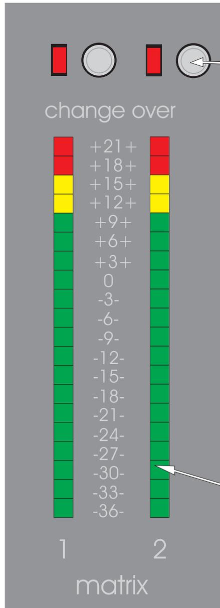
The CHANGE OVER switches change the function of the left and right meters so that they monitor the stereo aux send outputs in place of the matrix outputs.
