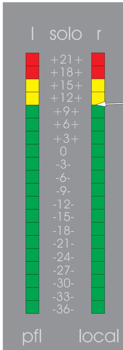
The meters monitor the peak signal level of the stereo AFL left and right solo busses or the PFL and local output level. The change over is automatic as part of the PFL Monitor switch on the COMMS module.
