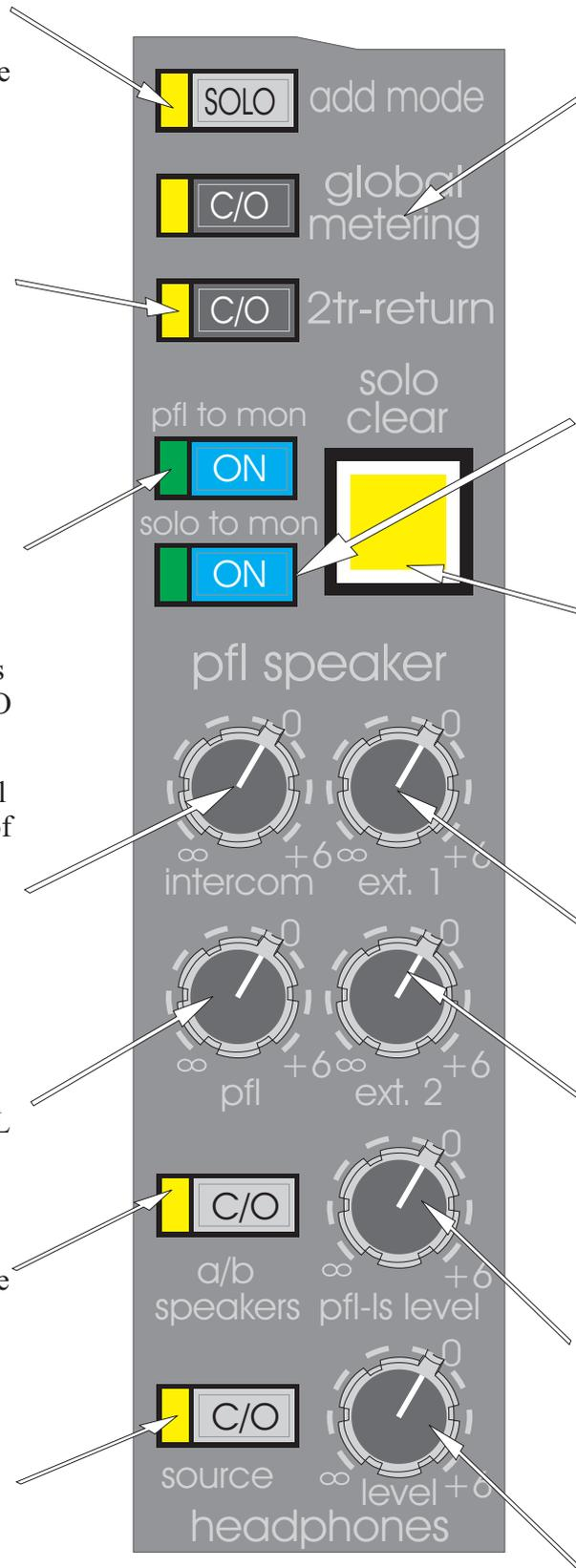
The GLOBAL METER CHANGE OVER switch changes the operation of every meter on the console except the comms meters and the record meters. The "normal" meter operation is to monitor pre fader on input channels and post fader on all other signals. When the global meter change over is active the meters change to monitor input amplifiers or bus amplifiers (as appropriate) on all signals.
