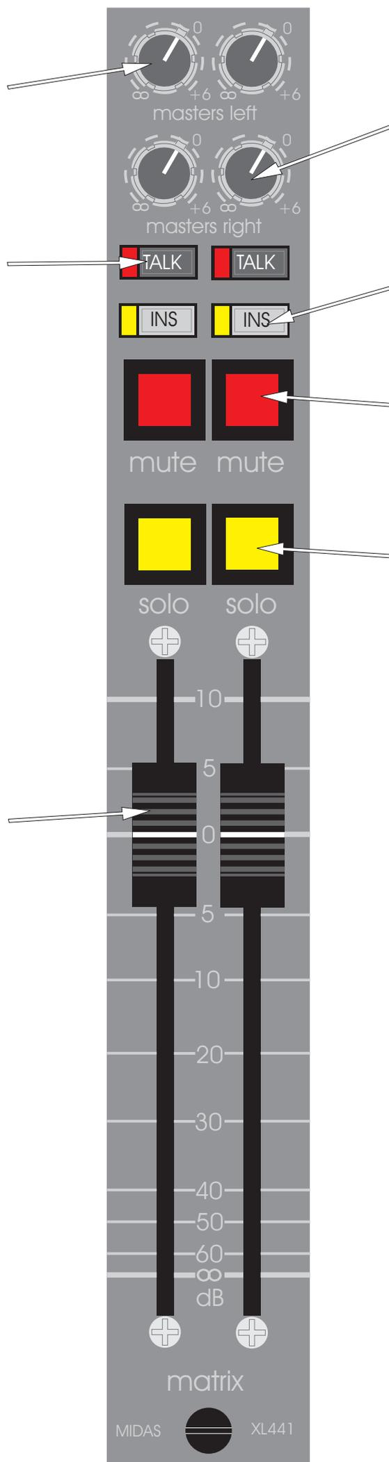
The MASTER RIGHT controls give continuous adjustment of master right signals that are sent to the matrix mixes. The adjustment is from +6dB to off.
