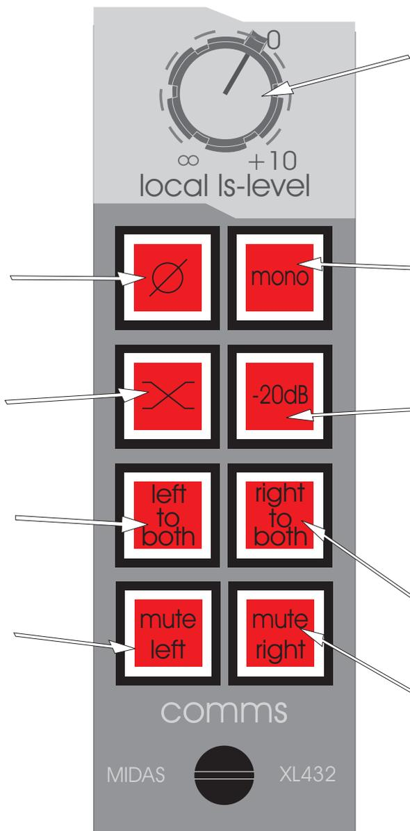
The LOCAL LS LEVEL control gives continuous adjustment of signals sent to the "A" or "B" monitor speaker outputs and has a range from +10dB to off.
