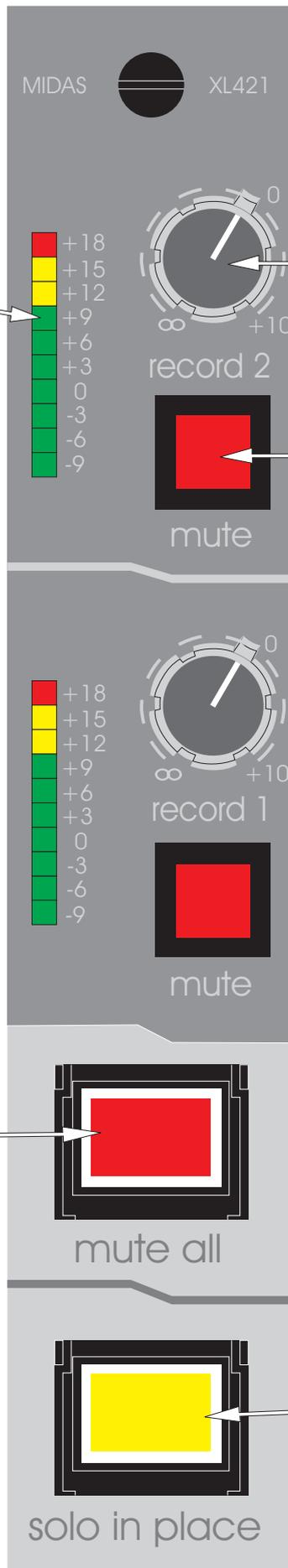
The RECORD controls ( 1 and 2 ) give continuous adjustment of the stereo record outputs from + 10dB to off. The record signals are derived from the pre insert master left and right signals.
