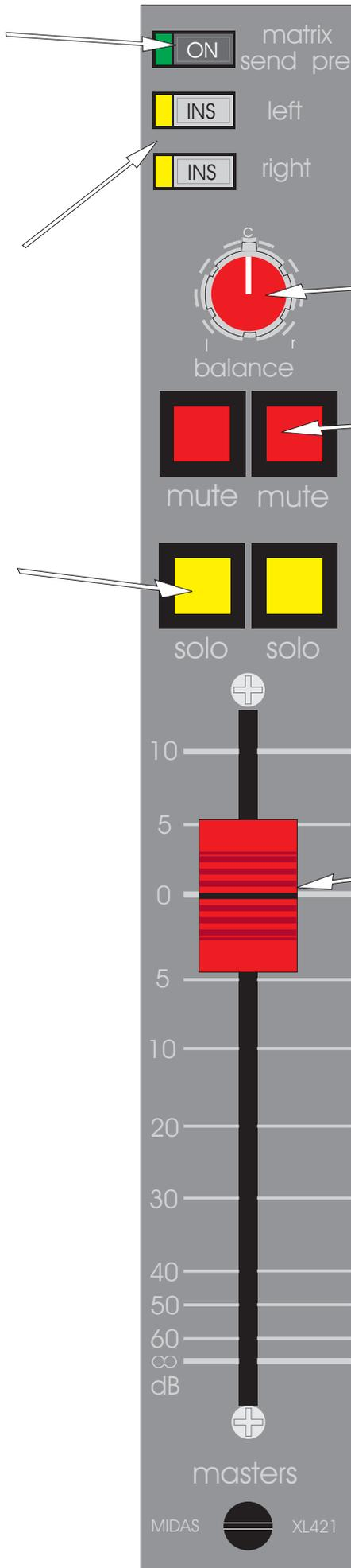
The BALANCE (pan) control gives continuous and reciprocal adjustment of the stereo left and right signal levels by + 3dB to off. This allows fine adjustment of the left, right power levels and imaging.
