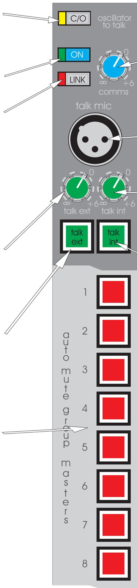
The COMMS control gives continuous adjustment of the incoming "clearcom" signals that feed to the headset and has a range from +6dB to off.
