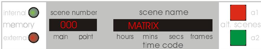
Scroll to MATRIX, Press CONFIRM, display prompts 000 SETUP, press CONFIRM
