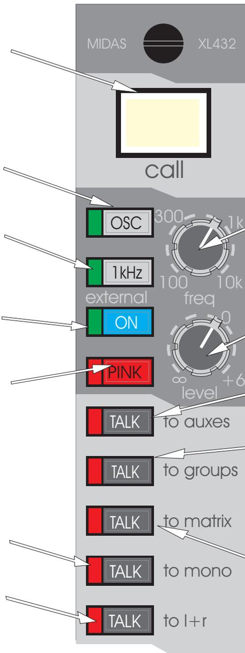
The FREQ control gives continuous adjustment of the oscillator frequency from 100Hz to 10K.
