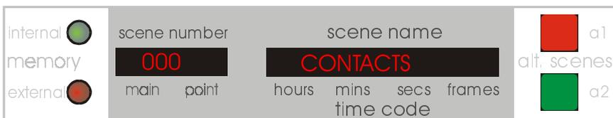
Scroll to CONTACTS, Press CONFIRM, display prompts 000 SETUP, press CONFIRM
