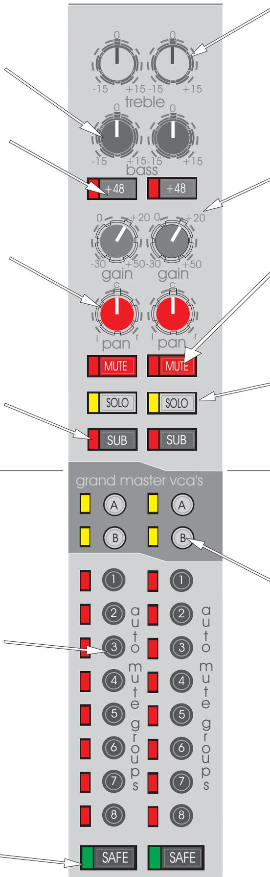
The TREBLE controls give continuous adjustment of boost and cut from +15dB to -15dB with a 0dB centre detent. The frequency is fixed at 10KHz.
