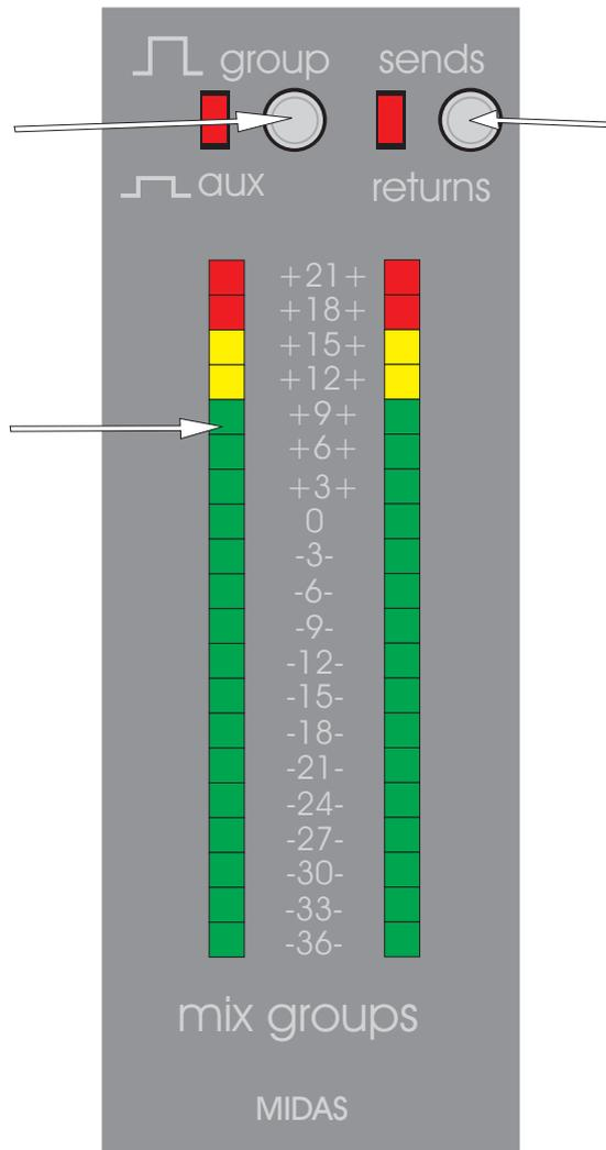
The RETURN switch changes the function of the left and right meters so that they monitor the post fader line return signals. If the AUX switch is not activated the meters return to monitoring the audio group outputs regardless of the RETURN switch position.
