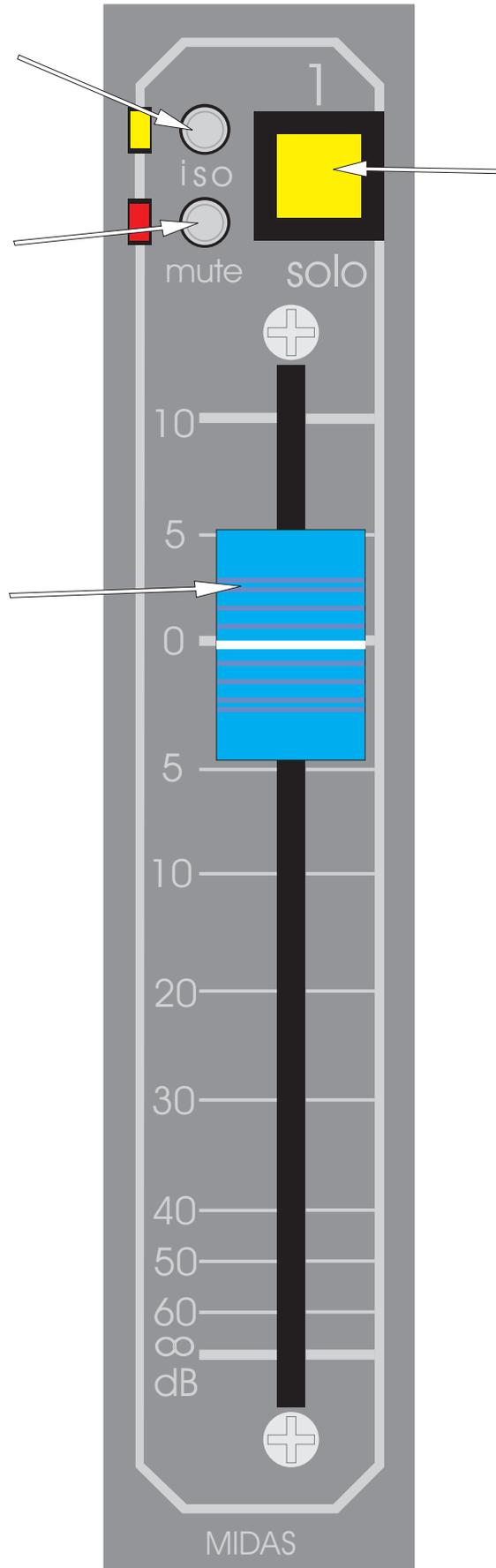
The vca SOLO switches are used to monitor VCA sub groups by creating a corresponding AUDIO sub group on the stereo AFL busses. All input channels and line returns that are assigned to a specific vca sub group will be summed onto the solo busses when that vca solo is active.
