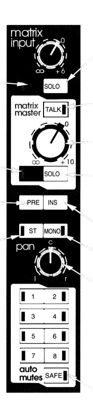
SOLO Solo's the Matrix signal to the main monitors (headphones or loudspeakers), with flashing LED indication.
