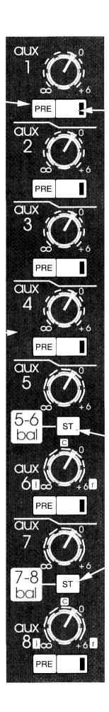
ON. Enables each auxiliary to send via it's rotary control with status LED.
