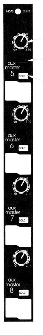
AUX MASTER 5-8 Adjusts the level of the auxiliary 5-8 Master output signal.
