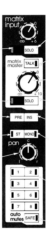
SOLO Solo's the Matrix signal to the main monitors (headphones or loudspeakers), with flashing led indication.
