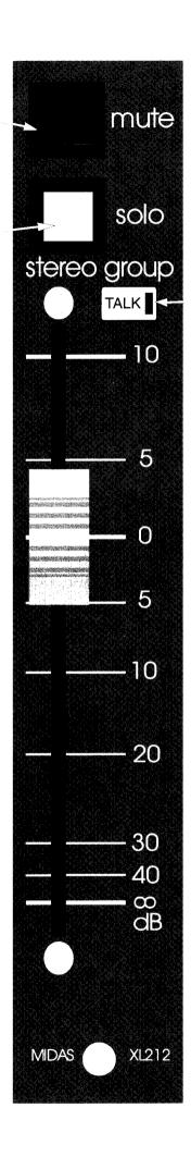
TALK Enables talkback signals to be routed to the Group output when the talk/generator system is used, with LED indication.
