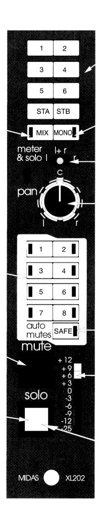
AUDIO GROUP ASSIGNS. Switches 1-6 route the input channel to the six mono audio sub groups. The left channel routing to odd groups (1,3,5) and the right channel routing to even groups (2,4,6). Switches STA and STB route the input channel in stereo to either of the stereo audio sub groups.
