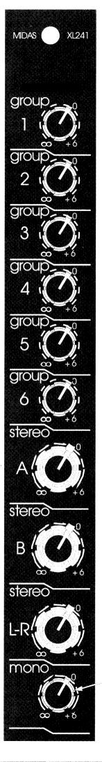
Adjusts the post-fader level of the Group 1 signal to the Matrix. Similarly, 2-6 controls Group signals 2-6.
