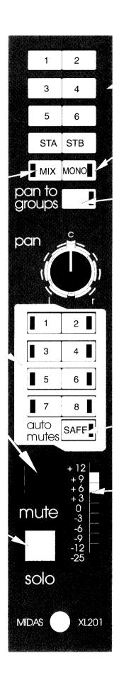
AUDIO GROUP ASSIGNS Switches 1-6 route an input channel to any of the six mono audio sub groups. Switches STA and STB route an input channel to either of the stereo audio sub groups.
