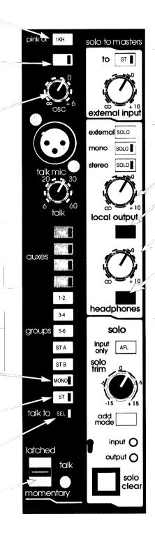
ST Connects the external input to the master left and right bus. EXTERNAL INPUT LEVEL Adjusts the level of the External Input.
