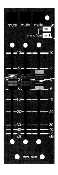
PRE Allows the signal feed from the main Left/Right outputs to the Mono output to be pre-fader rather than post-fader.
