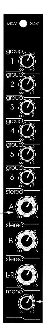
Adjusts the level of the post-fader Group 1 signal input to the Matrix. Similarly for Controls 2-6 for Group signals 2 to 6.
