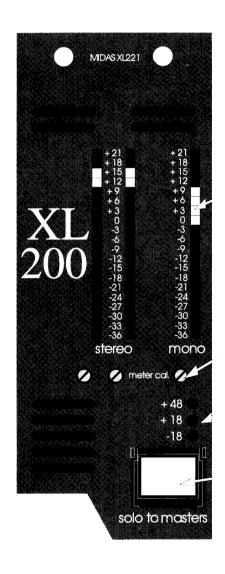
MONITOR METERS Three meters indicate left, right and mono, solo and PFL levels.
