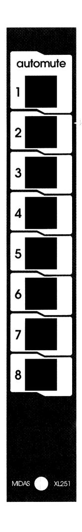
AUTOMUTES 1-8 The Auto Mute switches (1 to 8) activate the mute circuits on any assigned input channel or group
