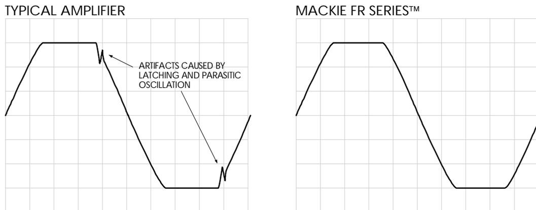
Mackie's Fast Recovery design recovers from clipping quickly without generating any undesirable artifacts. This performance is achieved by two unique design elements; the *Full Symmetry Dual Differential* front end provides excellent linearity while minimizing the need for negative feedback, and the *Baker Clamp* prevents output/driver device saturation. How these circuits operate is covered in depth in the circuit theory section.
