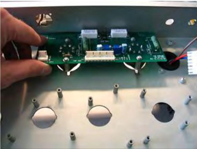
On opposite face of CHASSIS, finger tighten four (4) SCREWS as shown.
