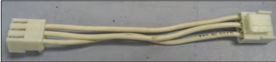
Connect the CABLE ASSY from the 'DIGITAL BOARD H12' header on the PCBA POWER SUPPLY to the POWER header on the PCBA MAIN.
