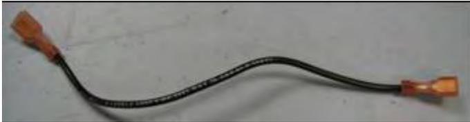
Connect the smaller spade on the CABLE ASSY to the bottom tab on the A/C RECEPTACLE. Connect the larger spade on the CABLE ASSY to the middle, top lug on the bottom TOGGLE SWITCH as shown.
