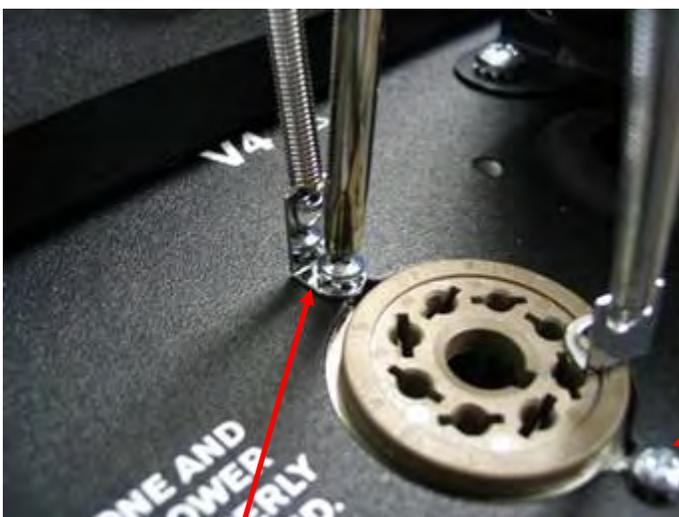
This screw shall be secure while installing **RETAINER** leg on opposite side
