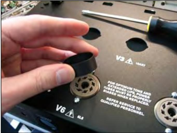
With the sleeve installed, tighten each SCREW to 6-8 in-lbs. After screws are fully tightened, remove the sleeve.
