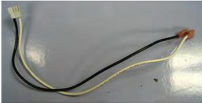
Connect the single black wire and single white wire as shown to the bottom TOGGLE SWITCH.
