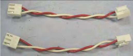
Connect one CABLE ASSY from the H2 header on the PCBA SPEAKER OUTS to the SPKR GND H8 header on the PCBA PRE-AMP.
