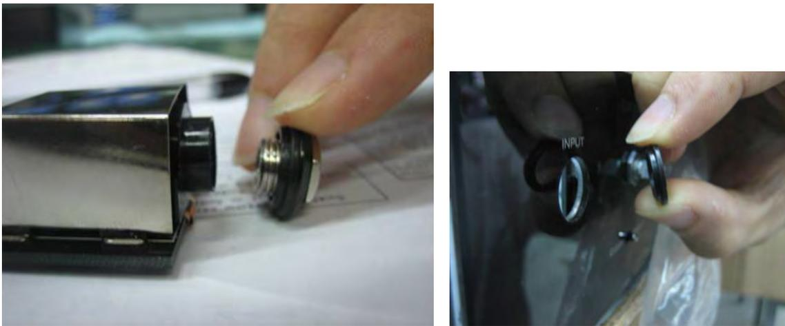
Note the alignment of the PCBA with the chassis. The tab on the PCB should align with hole in the chassis.
