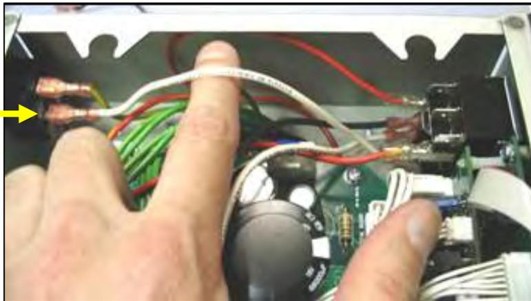
Connect smaller spade to middle tab on A/C RECEPTACLE
