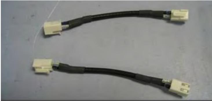
Connect one CABLE ASSY from the “H6” header on the PCBA GUITAR INPUT to the GUITAR “H2” header on the PCBA PRE-AMP as shown.
