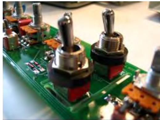
Breakaway the toggle switch PCB from the PCBA ANALOG U/I as shown.
