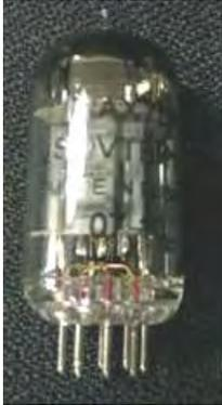
Install the TUBE in the indicated location (V4). Press firmly until the TUBE is fully seated.
