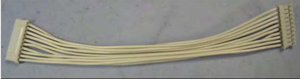
Connect the CABLE ASSY from the “H1” header on the PCBA DIGITAL U/I to the “H10” header on the PCBA MAIN as shown.
