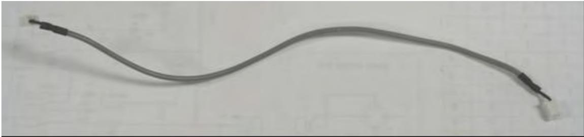
Connect the CABLE ASSY from the AMP FX RTN “H5” header on the PCBA DIGITAL U/I to the VDR “H6” header on the PCBA PRE-AMP as shown.
