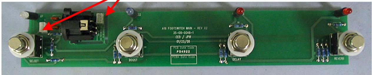
3. **BREAKAWAY BOARD:** Do not break apart breakaway board until installation in the chassis.
