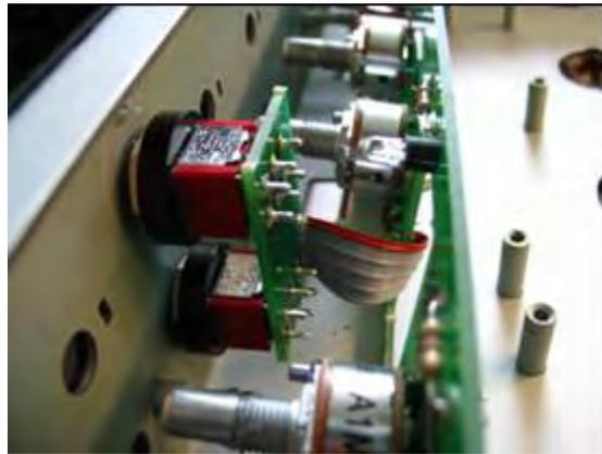
Verify that CAPACITOR C3 on the PCBA ANALOG U/I is bent down as shown. The PCBA will not assemble into the CHASSIS unless CAPACITOR is bent down as shown.
