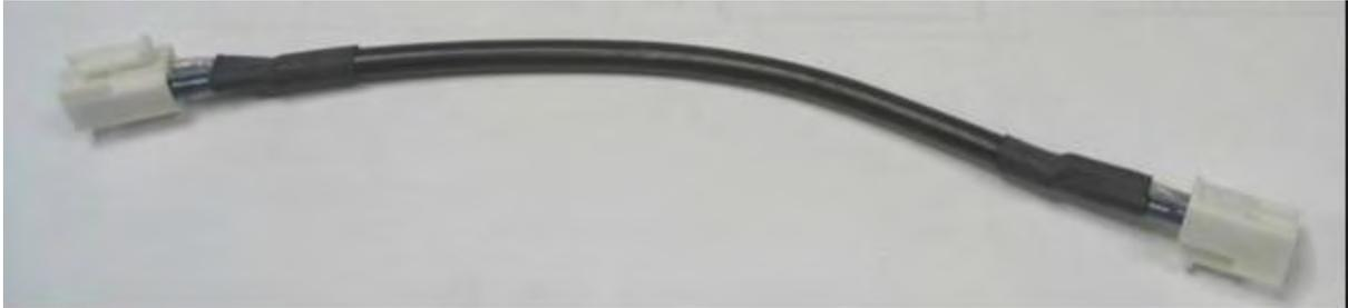
Connect the CABLE ASSY from the MV21 “H10” header on the PCBA ANALOG U/I to the ZMV2 “H10” header on the PCBA PRE-AMP as shown.
