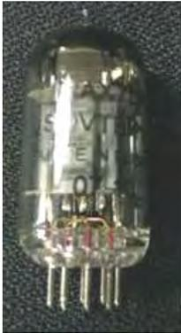
Install the TUBE in the indicated location (V5). Press firmly until the TUBE is fully seated.
