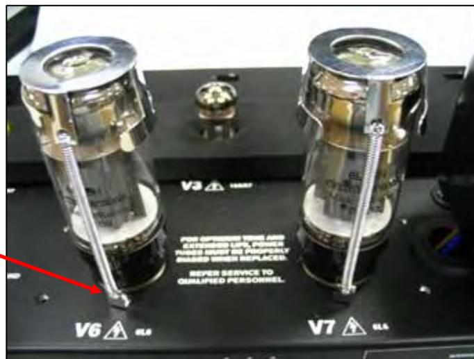
Ensure the SCREWS for the TUBE RETAINERS are still torqued to 6-8 in-lbs.
