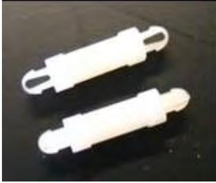
Insert one end of each DUAL LOCKING PCBA SUPPORT through the holes in the PCBAs.
