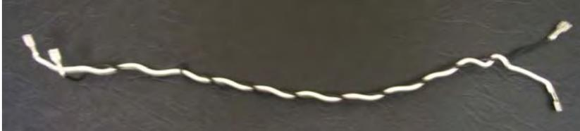
Plug the Fast-on connectors from the SPEAKER CABLE to each set of speaker lugs. Be sure to connect the correct wire to the correct lug.
