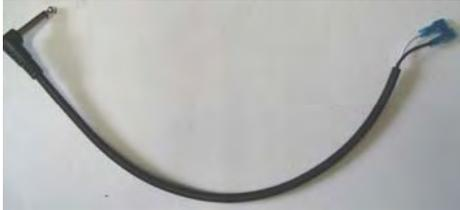
Plug the 1/4" plug from the SPEAKER CABLE into the 1/4" jack labeled "A" on the back panel of the CHASSIS.
