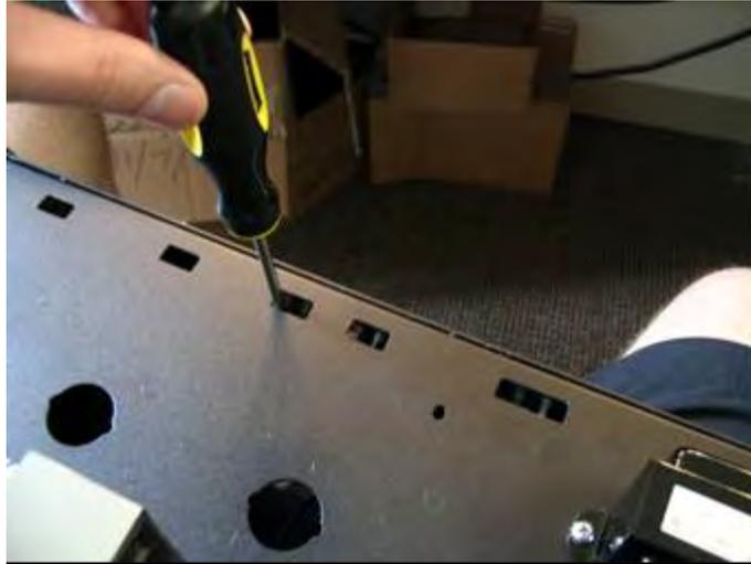
Secure each TOGGLE SWITCH to the CHASSIS and OVERLAY by tightening HEX NUTS. Torque each HEX NUT to 5-6 inch-pounds.
