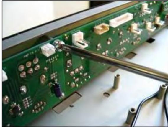
Install HEX NUTS over each POTENTIOMETER shaft as shown (3PL). Torque each HEX NUT to 5-6 inch-pounds.
