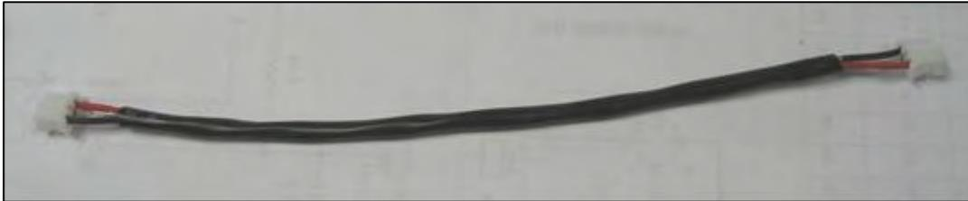
Connect the CABLE ASSY from the MV1 RTN/SND “H5” header on the PCBA ANALOG U/I to the MV1 “H19” header on the PCBA PRE-AMP as shown.
