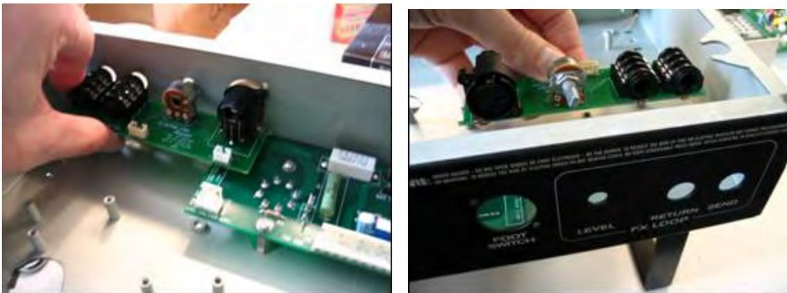
Install the WASHER and the HEX NUT over the POTENTIOMETER shaft as shown.
