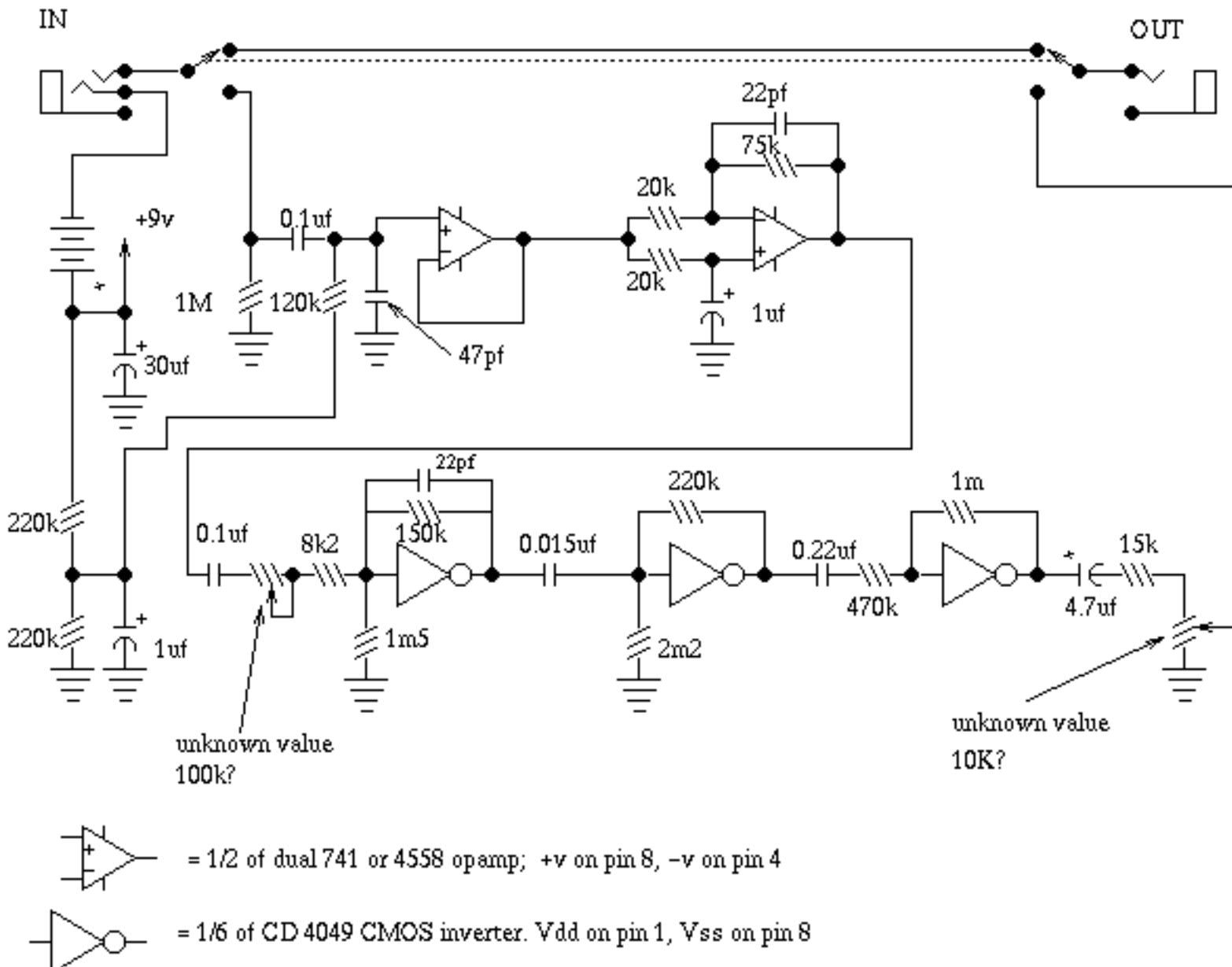
The MXR Hot Tubes is a commercial cousin of Craig Anderton's "Tube Sound Fuzz". It differs in that it uses a dual opamp input buffer, more stages, and more filtering. Also, there appears to be a DC offset in the bias points of two of the inverter/distortion stages.
