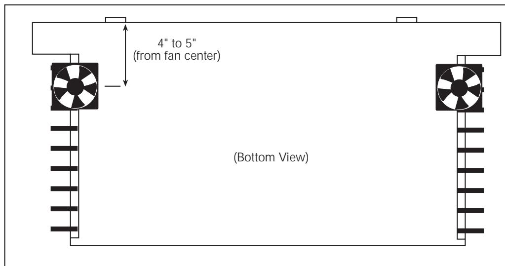
Fan center approximately in line with edge of unit and starting of heatsink fins
