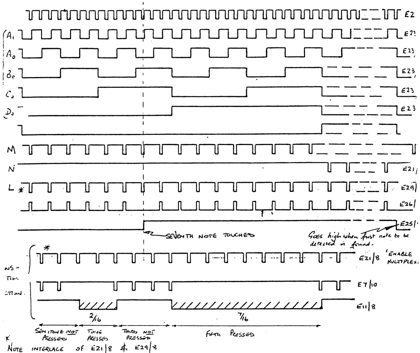
SIGNALS A1, A0, B0, C0 provide a four bit address code to the three data multiplexers. The top two multiplexers, E15, E27 are connected to the keyboard, and as only 30 notes are provided, then two inputs (E27 pins 7,8) are left permanently unconnected. The lower multiplexer is the "transposition pad" unit.
