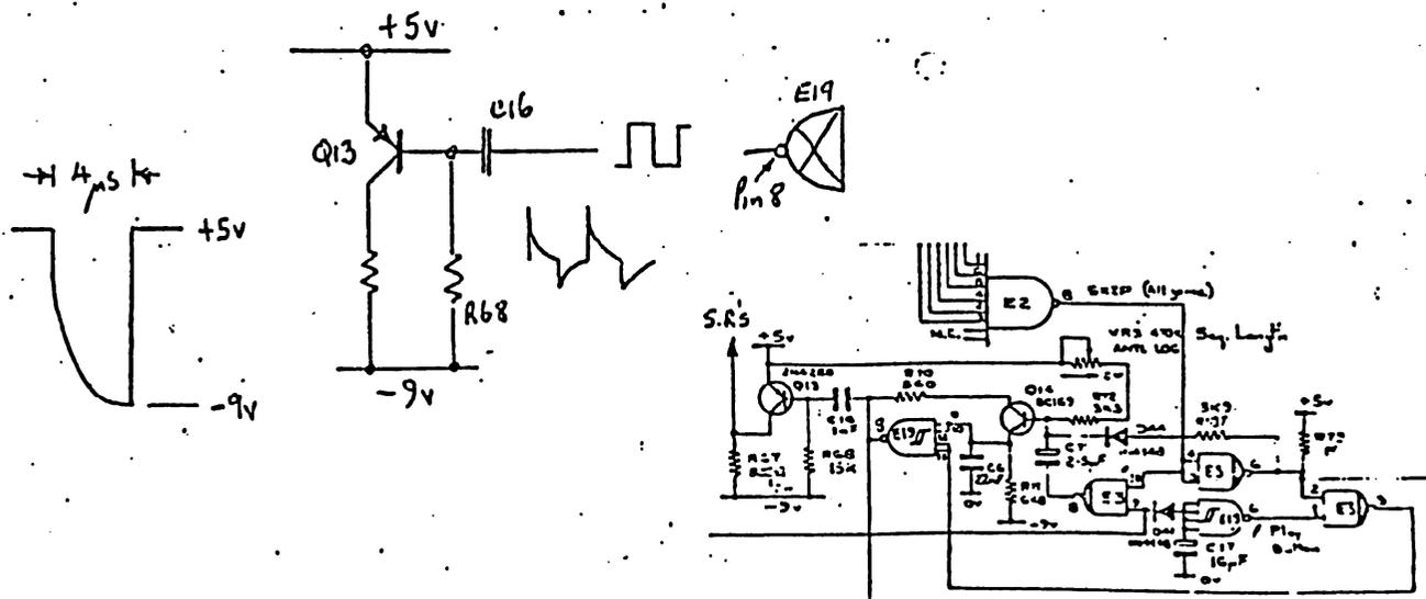
When the PLAY pad is pressed. Input pin 9, E3 goes low (but only for the duration of the pressing of the pad); this causes the data to rapidly recirculate (skip), usually for one bit only (because E3, 8 is high).
