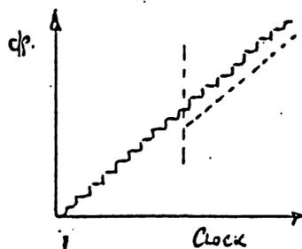
THE BIGGEST ERROR IN LINEARITY COMES 1/2 WAY WHERE A PRONOUNCED STEP CAN SOMETIMES OCCUR.
