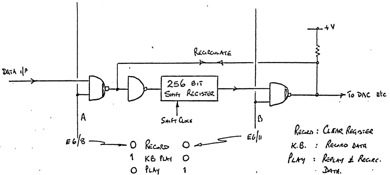
Lines A and B open and close the sets of input/output gates.
