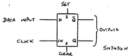
D type, used usually as a one bit delay or an edge detector.
