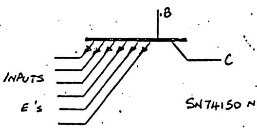
This is a multiple emitter, transistor, i.e. a transistor with, in this case, 6 emitters.
