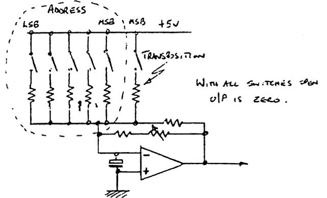
The switches are transistors Q7 and Q8-Q12 and the operation is similar to the real time DAC. Note, that the transposition acts only on the recorded output DAC, but no record of transposition playing is stored in the memory. Transposition is real time only.
