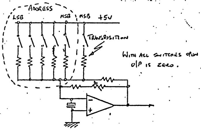
The switches are transistors Q7 and Q8-Q12 and the operation is similar to the real time DAC. Note, that the transposition acts only on the recorded output DAC, but no record of transposition playing is stored in the memory. Transposition is real time only.
