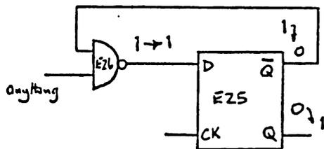
up, and it will remain latched up until it is released by a clearing pulse. Thus, E25, Q9 goes high and remains there when it detects the first note. (See page 2, waveforms). Now, E25, Q9 clocks the D types E16,17,18, which are fed with the address code (A, A<sub>0</sub>, B<sub>0</sub>, D<sub>0</sub>). So, as soon as the first note is detected, its address is clocked into E16,17,18 which act as a one bit memory. At the end of one address
