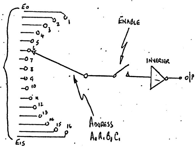
The 16 inputs; E0 to E15, can be considered as the 16 inputs to a rotary switch. The switch position (only one pole) is determined by the address code, ie A0, A1, B1, C1, labelled ABCD on the actual device.
