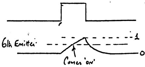
looking at the last trace we see that sixth emitter, which is connected to the touch plate, is dragged up, due to the associated capacitance of itself WRT its sister emitters. Infact, it is dragged
