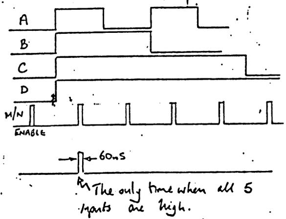
For each specific input there will only be one point in the Address cycle (32 bits) when all 5 emitters are high at the same time. When the bias is correctly aligned, the circuit will behave as follows:-
