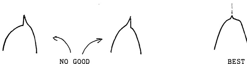
The best position is shown, where the small spike is triangular and balanced. A small thin spike may also appear but is not important.
