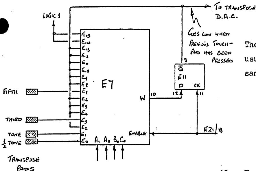
The multiplexer is addressed in the usual way, and is enabled and has the same touch sensitivity as before.
