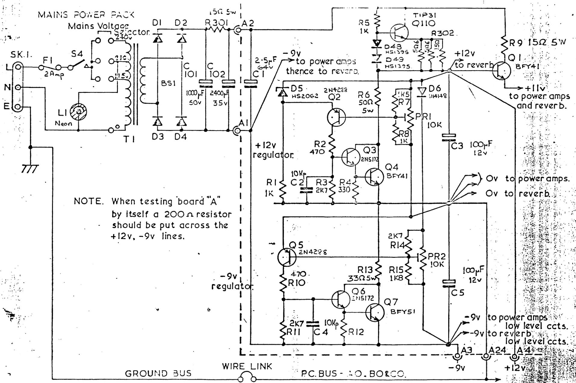
NOTE. When testing board "A" by itself a 200Ω resistor should be put across the +12v, -9v lines.
