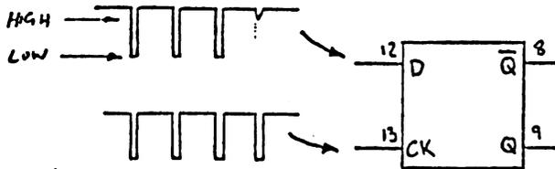
The D type operates as follows. It is an edge triggered device; that is data at its' D input is transferred to the Q output on the +ve transition of the clock. That is, put a 1 on
