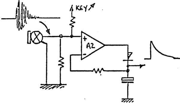
The network is a voltage follower with a diode in the feedback loop. The junction between the diode and the capacitor tries to follow the +ve voltage transient of the input and decays slowly (due to the storage of the capacitor) after the signal has
