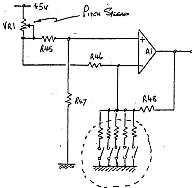
Inside the dotted box are 5 resistors and 5 switches. The resistors are R49 to R54, 1% m.o. resistors. The switches are Q1 to 5 and these are controlled by the stored address in E16, 17, 18.
