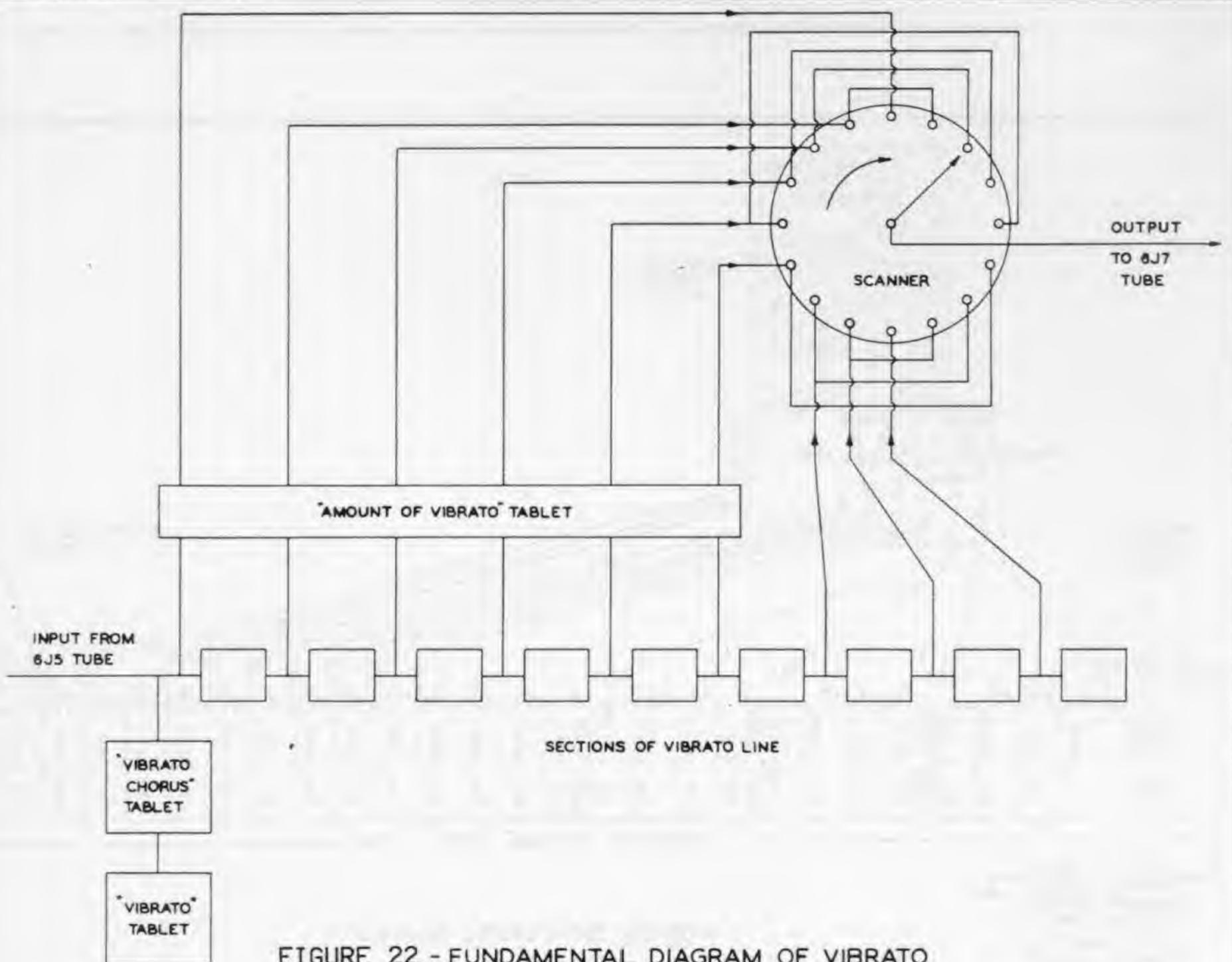
FIGURE 22 - FUNDAMENTAL DIAGRAM OF VIBRATO SYSTEM IN MODEL M ORGAN
