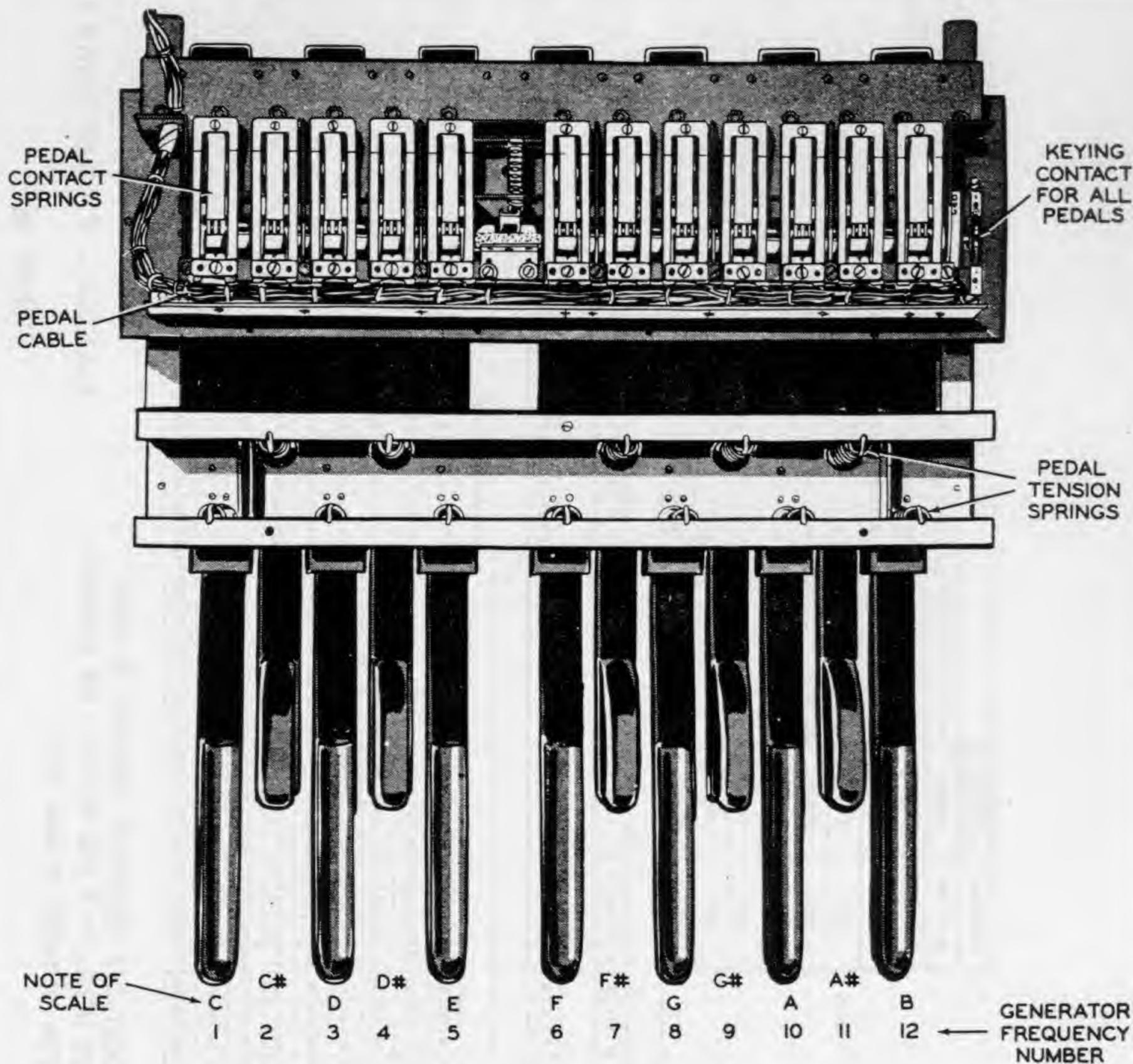
PEDAL KEYBOARD — MODEL M, M-2, AND M-3
