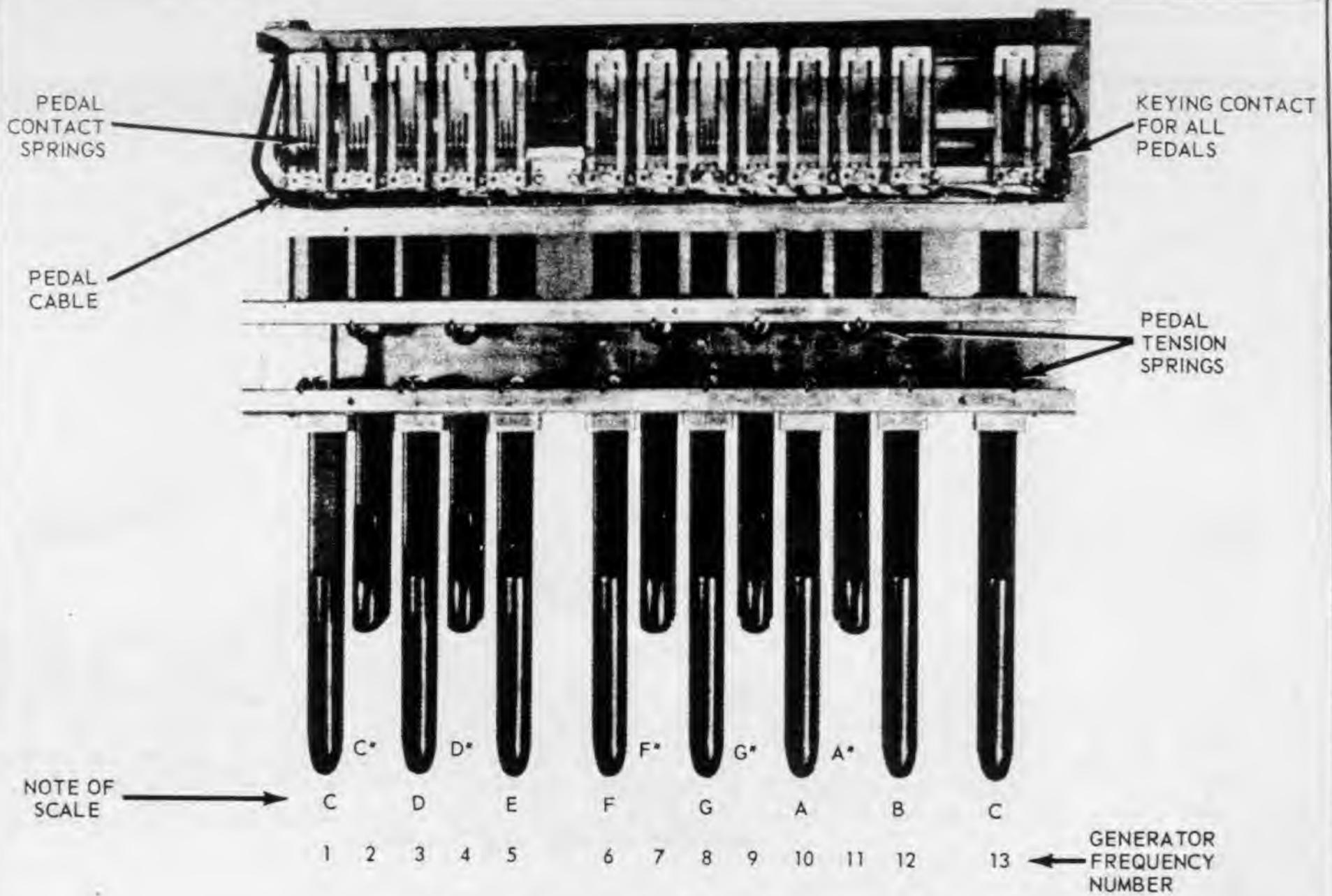
FIGURE 21. PEDAL KEY BOARD MODEL M-100
