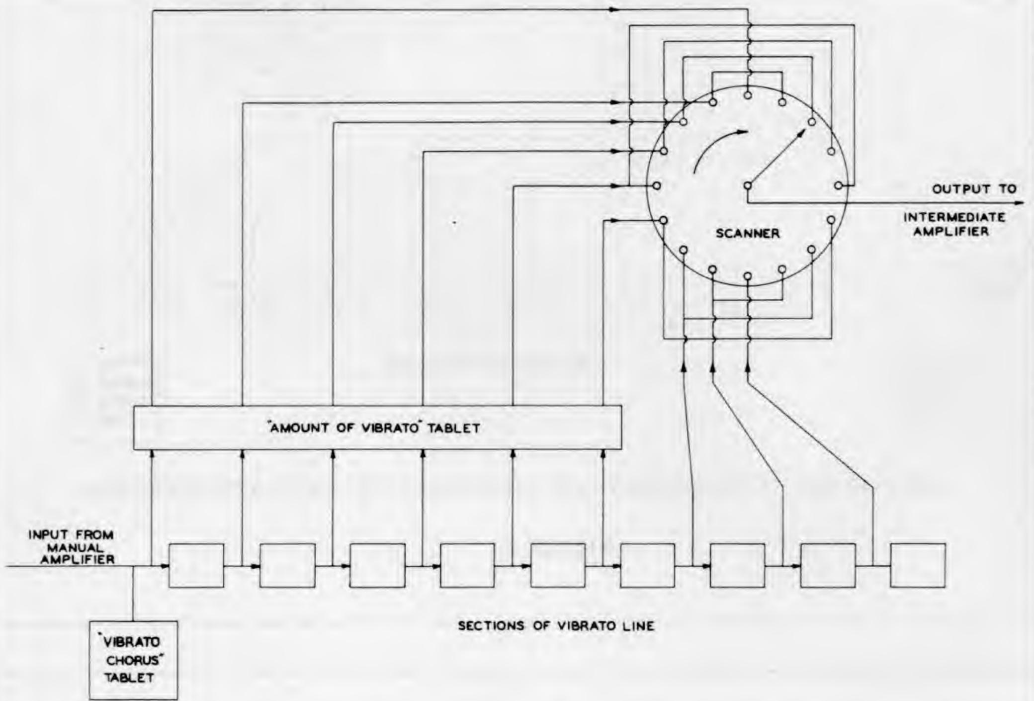
FIGURE 25 -FUNDAMENTAL DIAGRAM OF VIBRATO SYSTEM IN MODEL M-2 AND M-3
