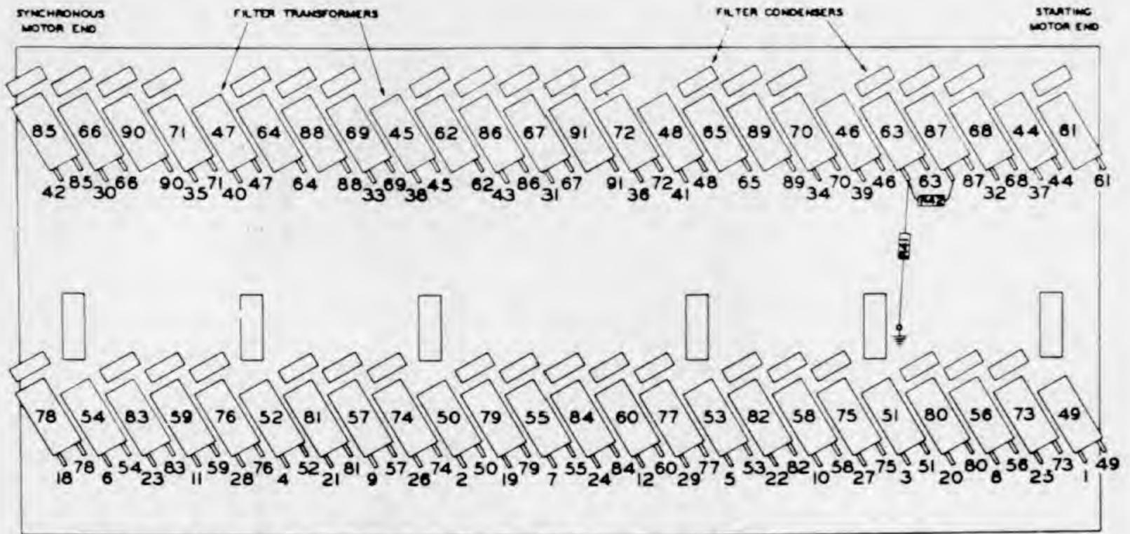
NUMBERS ON FILTER TRANSFORMERS ARE FREQUENCY NUMBERS OF TRANSFORMERS
