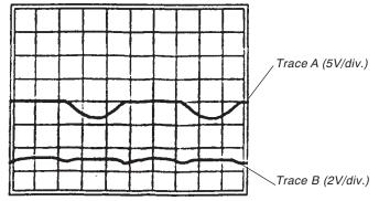
Solder the pins A-B of J16: the CH2 trace becomes continuous. Increase the generator level for the max. displacement of the CH2 trace toward the centre of the screen *Fig 7 Trace b*.
