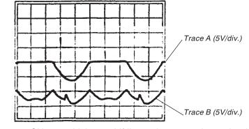
Set the scope CH2 sensitivity at 2V/div. and connect the probe tip at the testpoint TP3.
