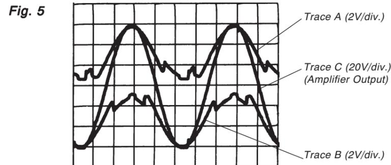
Disconnect the fan; wait until the temperature is 90°C (require some minutes) then decrease the input to zero. Adjust the trimmers R20 and R40, until the scope traces go respectively at -2.2Vdc and +2.3Vdc; turn on the cooling fan and wait until the temperature goes down to 80°C; then turn it off.
