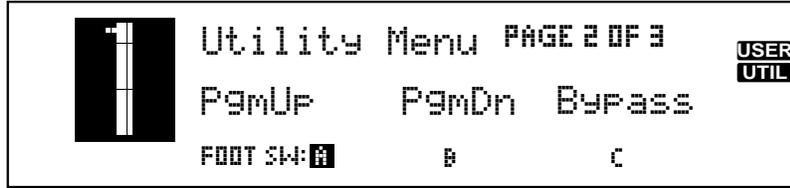
2. To make function assignments to any one of the three footswitches on the FS-300, press the **<Param 2>** button for switch A, press the **<Param 3>** button for switch B and press **<Param 4>** to select switch C.
