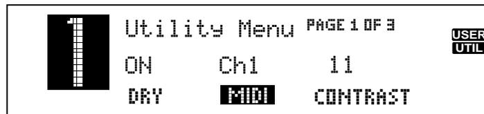
2. At this point, simply turn the <Program/Data> wheel to select the desired MIDI channel. The options for the MIDI channel selection ranges from: 1-16, ALL and Off.
