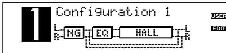
2. Now simply turn the <Program/Data> wheel until the desired configuration (1-5) appears in the display.
