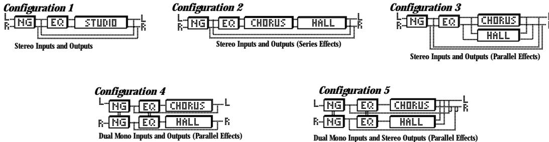
Effect Configuration 1 uses one effect module because both processing engines are combined for maximum processing power. This larger module allows you to have longer delay times and more dense sounding reverbs. Effect configurations 2-5 use Dual-Engine effect modules which allow you to use two effects per program.
