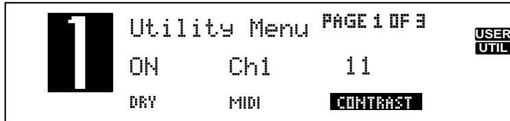
2. At this point, simply turn the <Program/Data> wheel to select the desired display contrast. To exit this or any other utility mode function, simply press the <Program> button.
