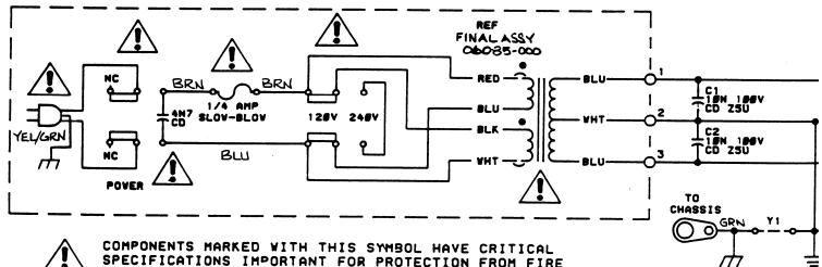
SPECIFICATIONS IMPORTANT FOR PROTECTION FROM FIRE AND ELECTRICAL SHOCK HAZARDS. WHEN SERVICING, IT IS ESSENTIAL THAT ONLY MANUFACTURER'S SPECIFIED PARTS BE USED FOR REPLACEMENT.
