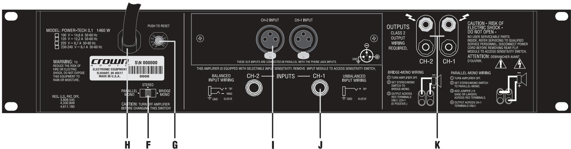
Figure 3.9 Power-Tech .1 Series Back Panel Controls and Connectors
