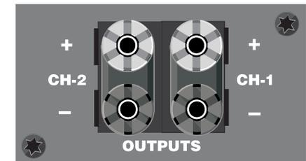
Figure 4.6 Model CEAS2 5-way Binding Post Output Connectors
