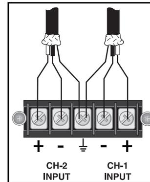
Figure 2.5 Barrier Strip Input Wiring: Balanced Signal In
