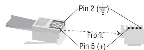
Figure 4.4 RJ-11 Jack Wiring and Pin Assignments
