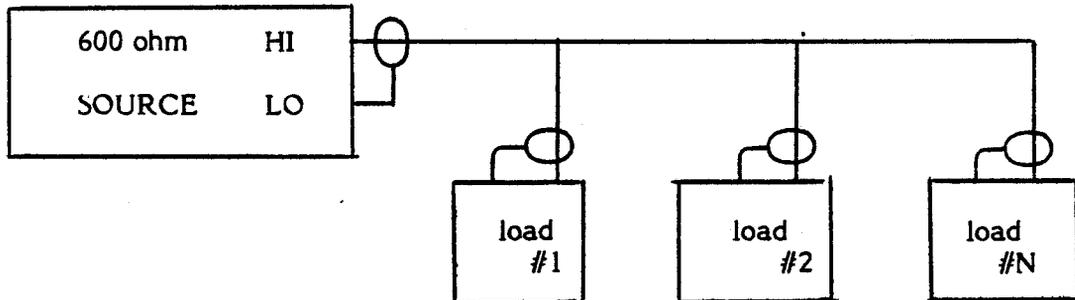
The Nth load should have a terminating resistor added to its octal plug between pin 1 and pin 6.
