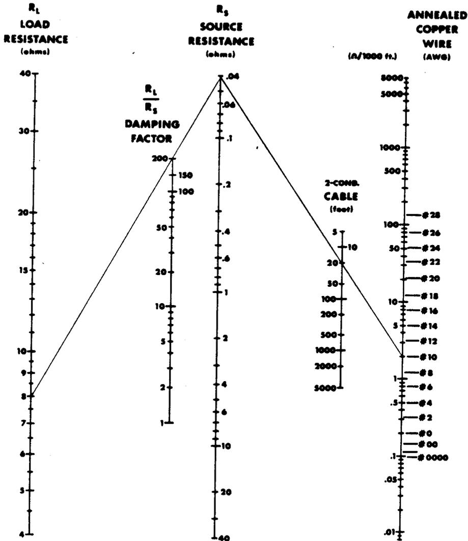
SOURCE RESISTANCE AND DAMPING FACTOR VS. LENGTH AND SIZE OF OUTPUT LEADS
