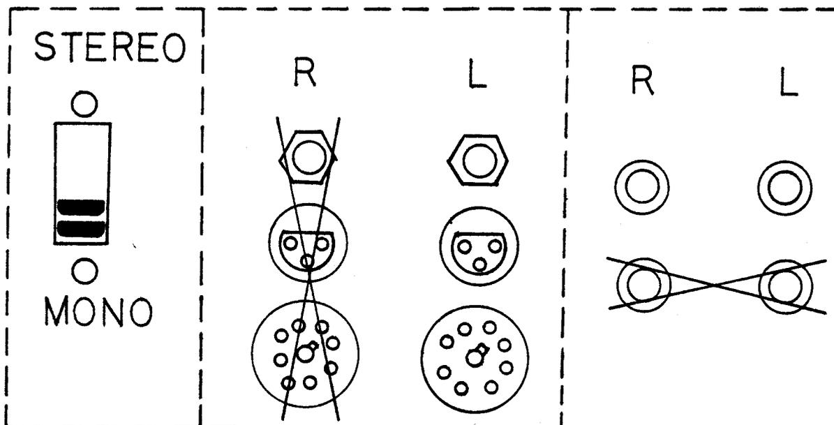
NOTE: Minimum load impedance for mono operation should be 8 ohms.
