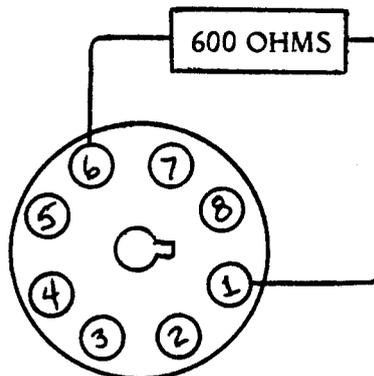
or by installing the resistor in a 1/4" phone plug and inserting it into the unused unbalanced input jack.
