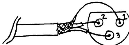
Note: Shield not connected to anything at signal source.
