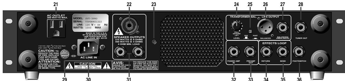
**21. AC OUTLET (DOMESTIC UNITS ONLY):** This unswitched outlet lets you connect any AC powered device (such as an effects unit or an electronic tuner) up to a maximum of 300 watts. The jack is "hot" whenever the amplifier is plugged into a live AC outlet, regardless of the setting of the amplifier's Power switch.
