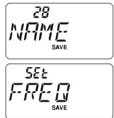
To display the alpha-numeric Tag again, just repeat the above procedure, rotating the **DIAL** knob to select “ALPHA” in step 5 above.
