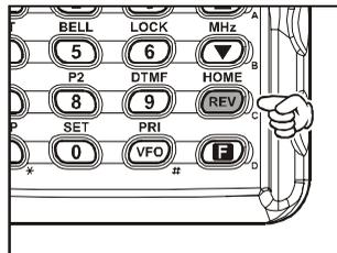
*The configuration of this key may be set either to “RV” (for checking the input frequency of a repeater), or “HM” (for instant switching to the “Home” channel for the band you are operating on). To change the configuration of this key, use Set Mode Item 33: REV/HM. See page 77.*
