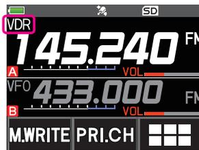
When a signal is received on the priority channel, the beep sounds, and the Dual Receive function stops temporarily.
