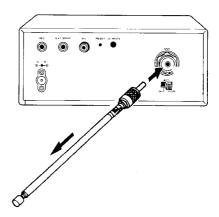
If it is necessary to use an external antenna other than the one supplied, use a wide-band antenna of 50 ohms or a special antenna designed for the specific frequency band to be received.
