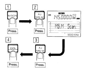
3. To remove a frequency from the list of frequencies used by the Memory-Scan Memory operation, use the following procedure.
