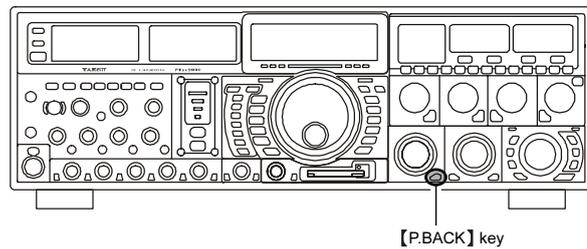
Pressing the **[P.BACK]** switch once more will halt the recording, and the LED imbedded in the switch will go out.
