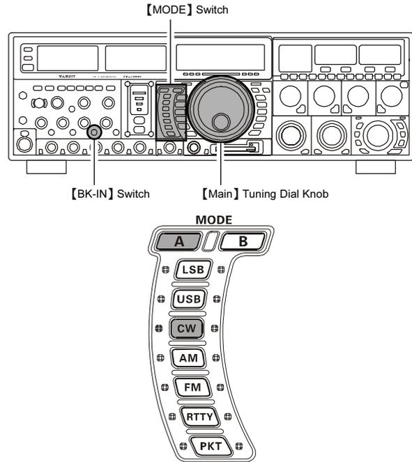
In the illustration, Figure A demonstrates the normal CW injection setup, using the USB side. In Figure B, CW Reverse has been engaged, so as to receive using LSB-side injection to eliminate interference.
