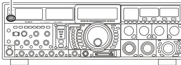
You may also customize the amount of brightness reduction engaged by the pressing of the **【DIM】** switch, and may use different brightness levels for different front panel areas. Menu item **[DISPLAY 014 DIMMER-METER]** adjusts the brightness level of the analog meters and the LCD display, while menu item **[DISPLAY 015 DIMMER-VFD]** sets the brightness levels of the main frequency display (these settings are effective only when the **【DIM】** switch is pressed).
