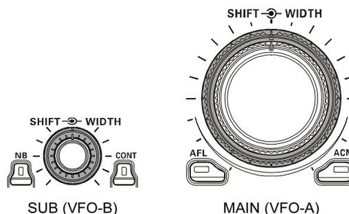
Referring to Figure (B), you can see the default bandwidth with the **[WIDTH]** control set to the 12 o'clock position.
