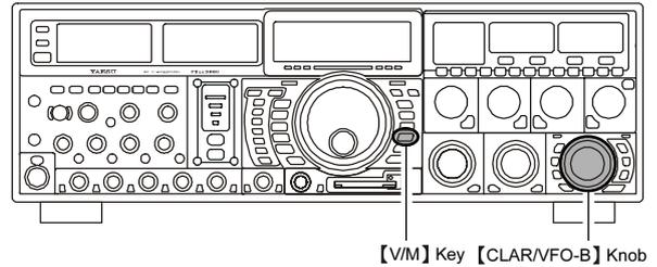
To operate on the 60-meter band channels, press the **[V/M]** key (#39), if necessary, to enter the Memory mode, then rotate **[CLAR/VFO-B]** knob (#97) to select the desired channel from the above selections.
