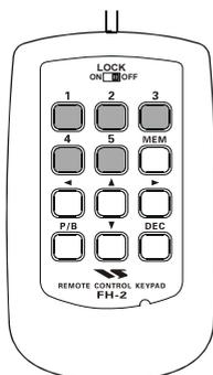
5. Use the FH-2's **[◀]** and **[▶]** keys to set the cursor position and use the **[▲]** and **[▼]** keys to choose the letter/number to be programmed in each slot of the memory. In the case of the second example above, the “}” character designates the slot where the Contest Number will appear.
