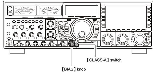
Clockwise rotation of the **[BIAS]** control increases the Bias, and fully clockwise rotation of the **[BIAS]** control will place the transmitter in fully Class-A operation. Counter-clockwise rotation of the **[BIAS]** control will move the transmitter toward Class AB operation.
