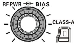
Clockwise rotation of the **[BIAS]** control increases the Bias, and fully clockwise rotation of the **[BIAS]** control will place the transmitter in fully Class-A operation. Counter-clockwise rotation of the **[BIAS]** control will move the transmitter toward Class AB operation.
