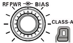
2. Engaging the "Class-A" mode actually places the transceiver in a condition whereby the Bias level may be adjusted, using the **[BIAS]** control (#66), to set the transceiver for operation anywhere between Class A and Class AB (which has lower heat dissipation but higher distortion products).
