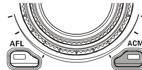
When ACM is turned on during Dual Receive operation, the audio from the Sub (VFO-B) receiver will disappear.
