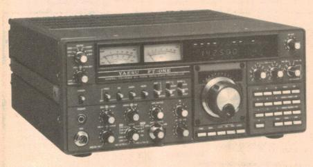
reads operating conditions selected by the meter switch (top left hand) while the inner meter indicates signal strength and ALC value. The bottom right hand corner is the computer processing unit (CPU) keyboard, which controls the operating frequency, scanning, and VFO selection. Under the tuning knob are the fine and fast tuning, clarifier and frequency lock switches.
