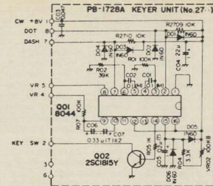
Fig. 7—The very neat, small optional keyer board available for the FT-One. The circuit is based on a Curtis 8044 Keyer IC.
