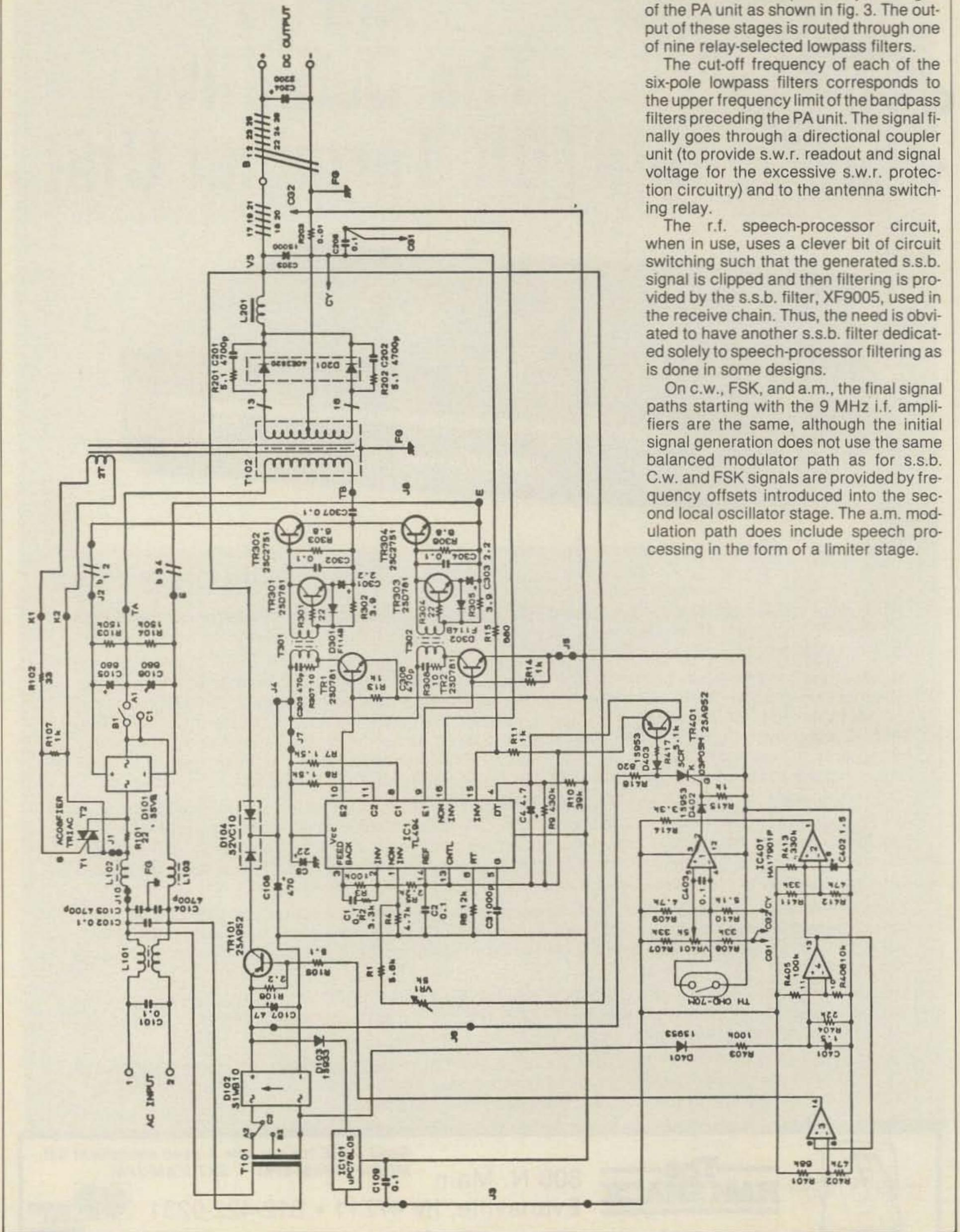
just the reverse of the signal flow path on receive. However, the low-level signal must now be amplified to the 100 watt level, and this is accomplished by the stages of the PA unit as shown in fig. 3. The output of these stages is routed through one of nine relay-selected lowpass filters.
