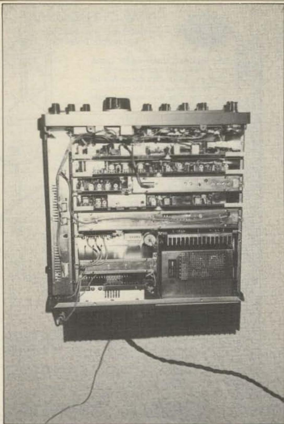
Taking the top cover off the transceiver, one sees an impressive assembly of large PC boards and shielded enclosures. The power-supply compartment is on the lower right, and the PA compartment is on the lower left. Normally one will have to take the top cover off once to reach various adjustments if one wants to tailor sidetone volume and pitch, AF monitor level, some VOX adjustments, etc., to individual preferences.
