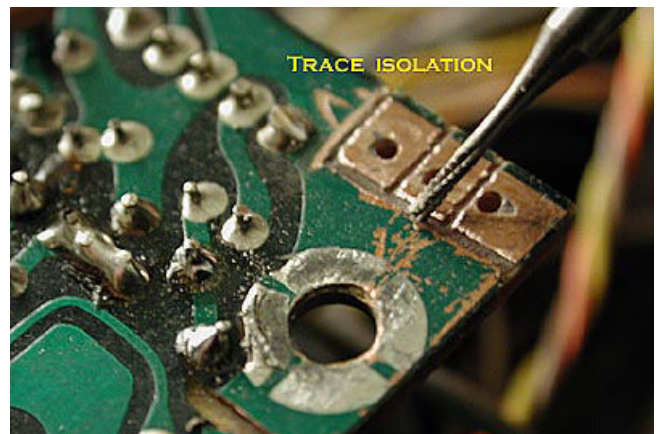
Figure 7 - Scrape away the copper between each hole to make a solder pad for each leg/terminal of the 7808.
