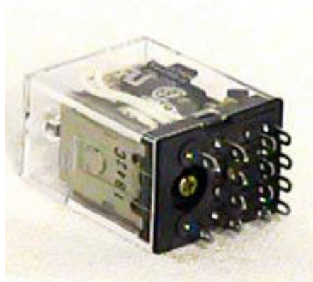
Main Chassis Relays RL1 & RL2 FRL263-DO12/04CS or Guardian Type 1315H (4PDT 5 AMP Contacts) Size: just over 1 cubic inch
