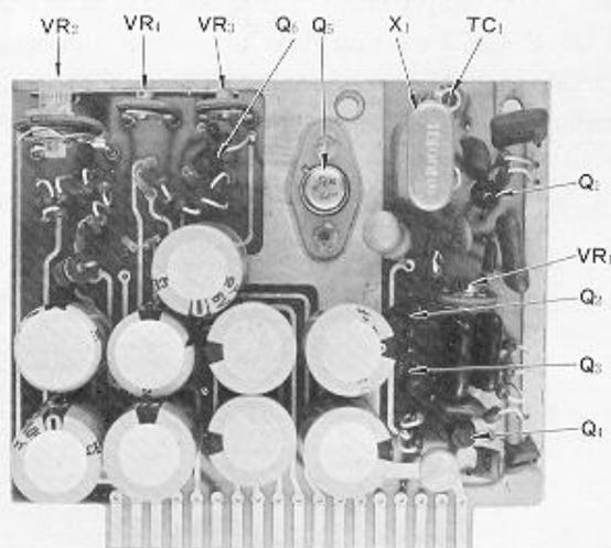
100 KHz against WWV or JJY. Output from the oscillator is fed to into 25 KHz multivibrator Q2 and Q3, 2SC735Y which generates a marker signal every 25 KHz. VR1 is used to synchronize the multivibrator to 25 KHz. The multivibrator operates when the supply voltage is applied through pin 17 from the switch on the front panel. The calibrator output is fed through the buffer amplifier Q4, 2SC735Y to the receiver antenna circuit from pin 16.
