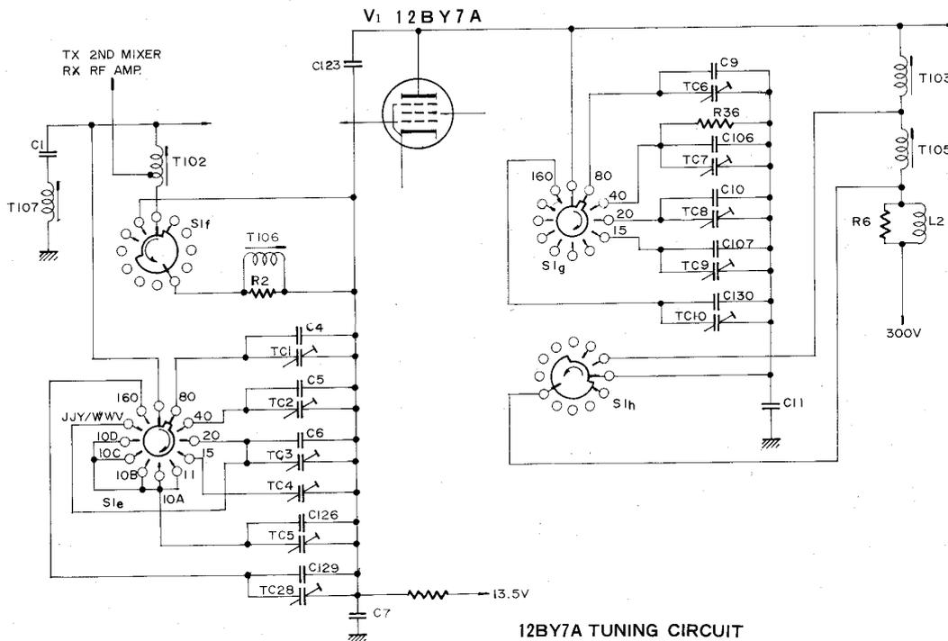
(9) Set the BAND switch at 80, VFO at 4,000 KHz, and the PRESELECTOR at 7 of the inner scale. Set TC1 and TC6 at the mid-capacitance point. Tune the transceiver to 4,000 KHz and adjust T105 and T106 for maximum transmitter power output into the load.
