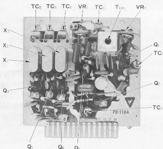
For AM and CW operation, the 3179.3 KHz crystal controlled oscillator Q6, 2SC372Y operates to produce the carrier signal, and Q3 and Q5 are disconnected.
