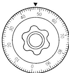
For bands 160-80-10B-10D read Red scale on main dial. Settings shown in the example would then read 648 KHz. For example, on 80 meters the frequency would be 3.648 MHz, on 10B, 28.648 MHz, etc.
