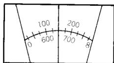
For bands 40-20-15-10A-10C read Black scale on main dial. Setting shown in the example would then be 148 KHz plus the starting band edge frequency in MHz. For example, on 40 meters the frequency would be 7.148 MHz. On 20 meters, 14.148 MHz, etc.
