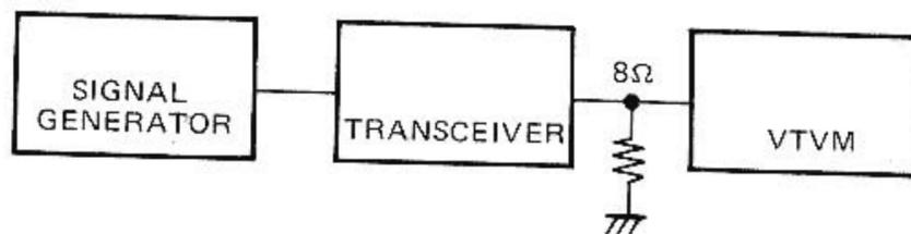
RX SENSITIVITY TEST SETUP
