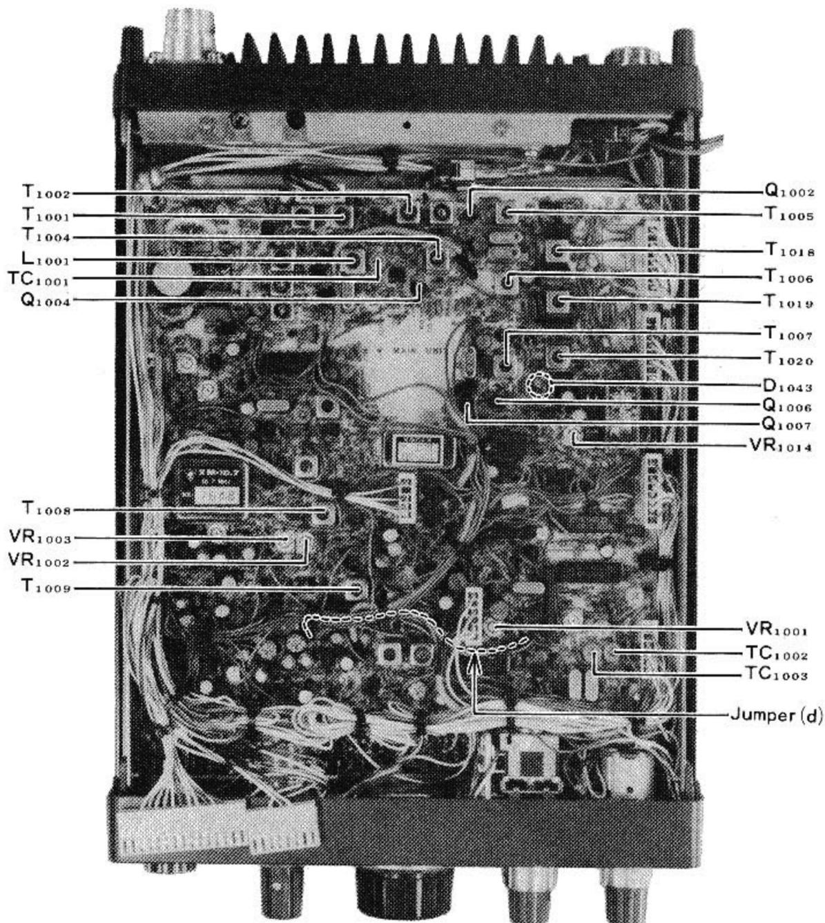
ALIGNMENT AND TEST POINTS FOR RECEIVER
