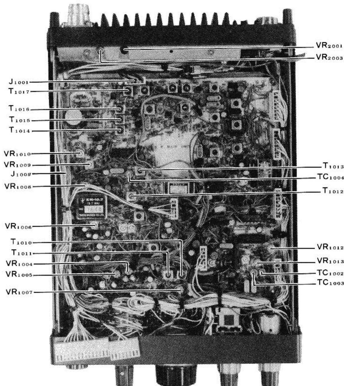
ALIGNMENT AND TEST POINTS FOR TRANSMITTER
