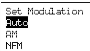
Select an item by turning [Scroll Control] until the item is highlighted, then pressing [E / yes / gps].
