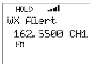
The scanner does not sound until it detects the 1050 Hz Weather Alert Tone or decodes the SAME data in Weather Alert Scan Hold. See: [\*Weather Alert Scan\*](#) for operation when it detects the 1050 Hz Weather Alert Tone or decodes the SAME data.
