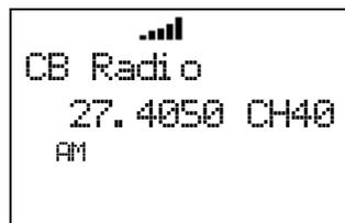
While monitoring the transmission, press [SCAN / srch] in Function Mode or turn [Scroll Control] to resume searching.
