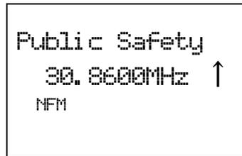
The Scanner starts from the lowest frequency of the selected range and searches in ascending or descending order. While searching, turn [Scroll Control] to change the searching direction.
