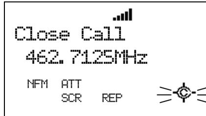
In this condition, the scanner does not check for other Close Call hits.
