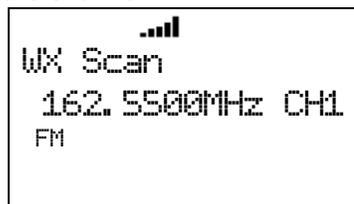
If the signal is lost, the scanner resumes scanning for Weather Channels.
