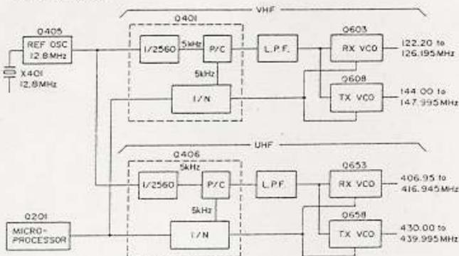
Figure 4-1 PLL Block Diagram
