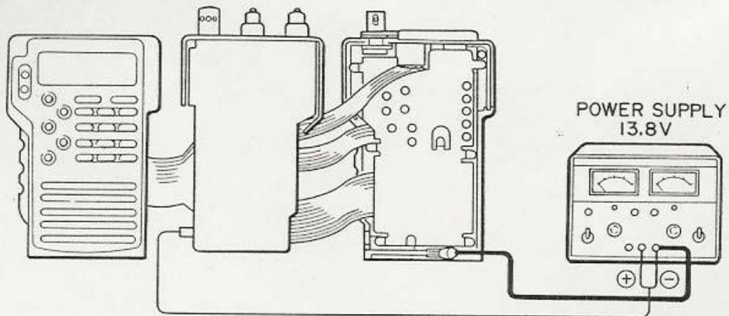
Figure 2-8 Ground cable running for transmit power alignment
