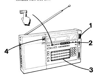
1 Keeping the PT1 key pressed, turn the TIME ADJ knob to set the turn-on time.
