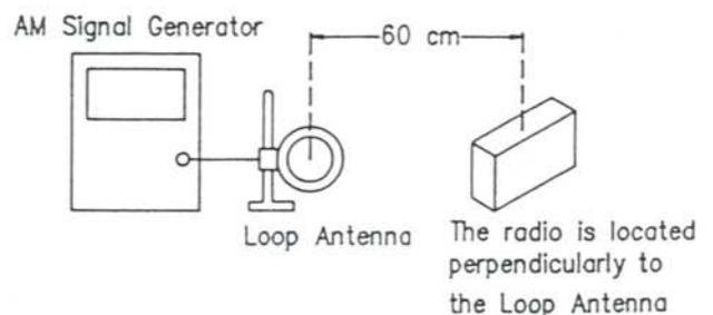
(10) ALIGNMENT FOR SIGNAL STRENGTH LEVEL
