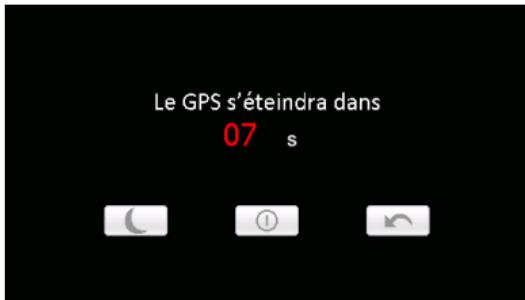
In this UI click the button will be in sleeping mode, click the button will power off ; click the button to exit the UI and back to normal operation.
