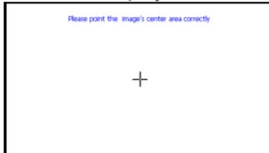
On this UI, use stylus to tap at the center of the cross, then tap on other crosses which will move after each tapping until finish and "Touch Screen Calibration Completed" is shown.
