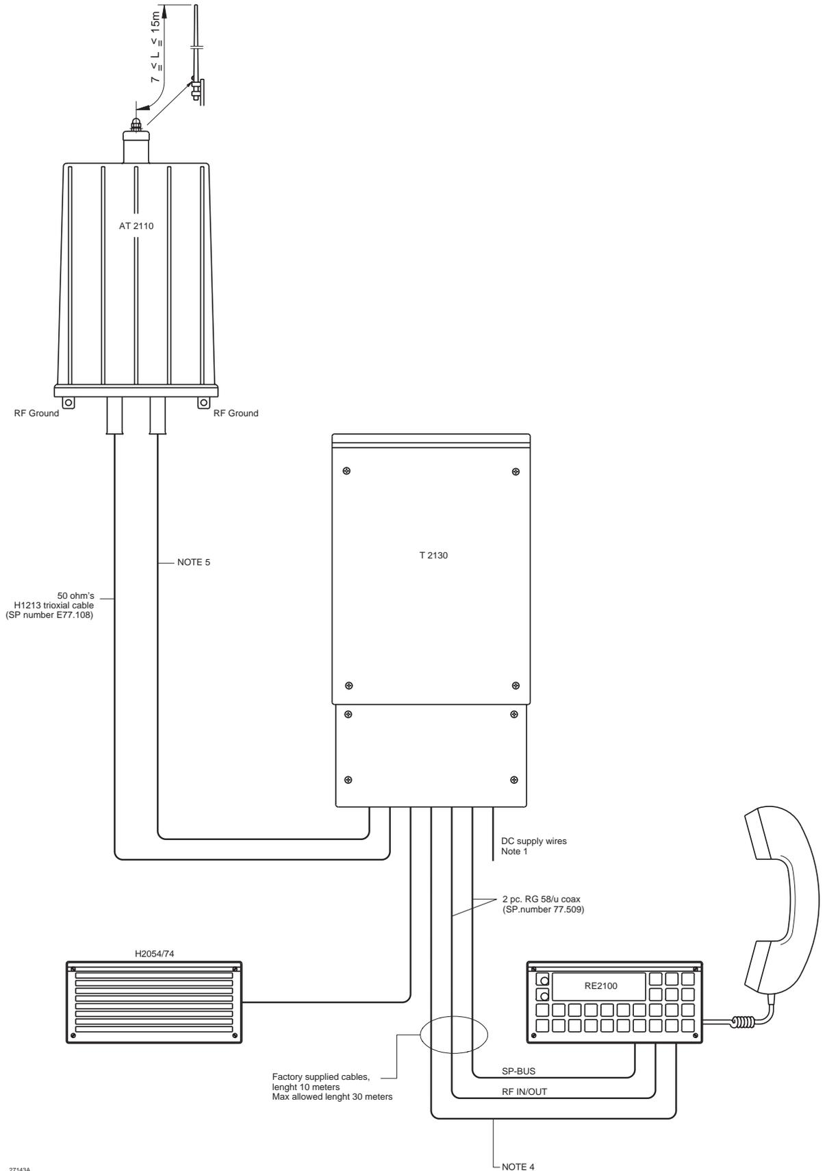
**2.2.5 MAIN CABLE PLANE WHEN SUPPLIED FROM 12V DC BATTERY, USING N2160 12V DC TO 24 V DC CONVERTER.**
