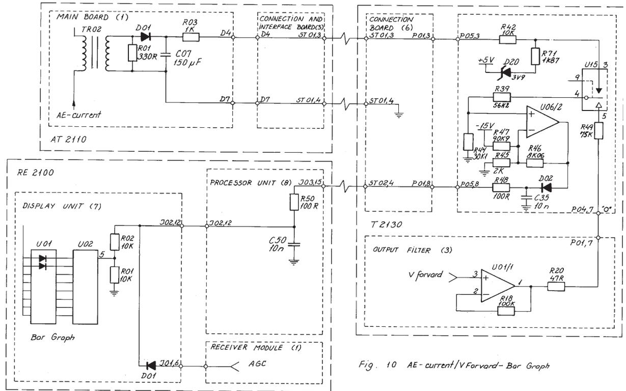
Fig. 10 AE-current/VForward- Bar Graph
