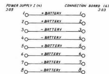
CABLE 5 : POWER SUPPLY I TO CONNECTION BOARD
