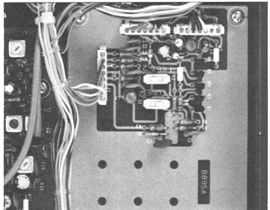
When S1 is set in the "2" position, the "START" terminal usually supplies about 8V DC through a 22K ohm resistor, and by pushing the TUNING SWITCH, the START terminal is grounded (0V) and sinks a current put out from the ANTENNA TUNER.
