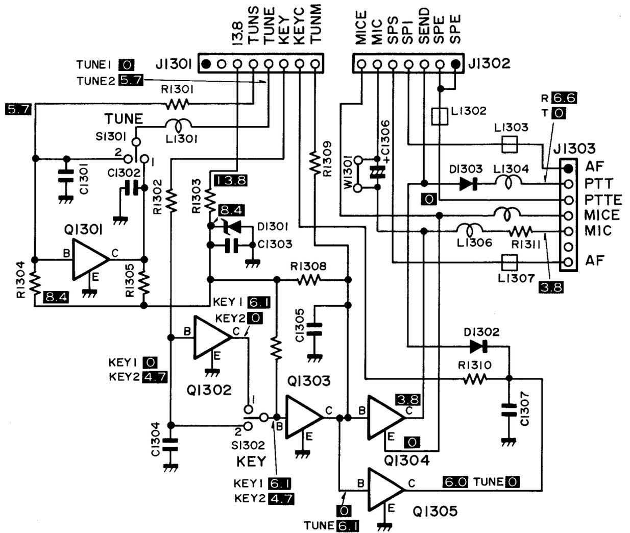
**4.0** DC Voltage by 50KΩ-V multimeter
