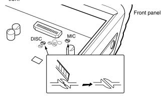
**NOTE:** Be sure to re-solder the above disconnected points when you remove the scrambler units. Otherwise no TX modulation or AF output is available.
