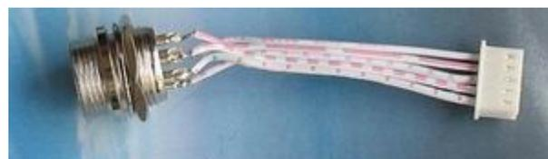
CN9: TX output. Connect to CN2 of PA board.
