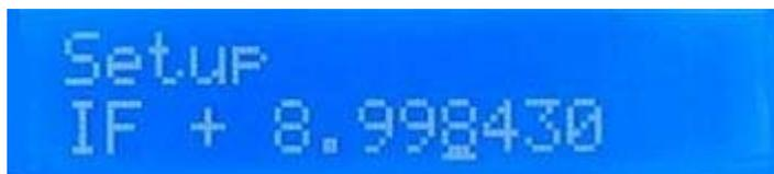
Set up the XTL filter offset. Press F+ and F- to set the above displayed data, +8.998430. The
