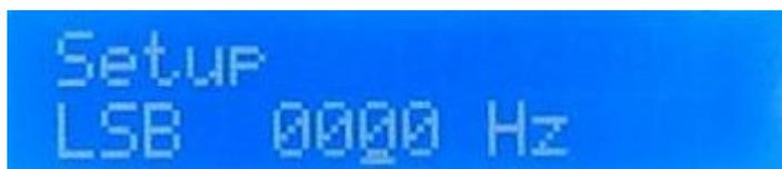
This is for setting up the LSB offset. Use the default value 0000. Press the IF SET again, and USB SETUP appears:
