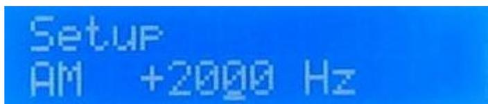
Set up the AM offset. Press F+ and F- to set the above displayed data, +2000.
