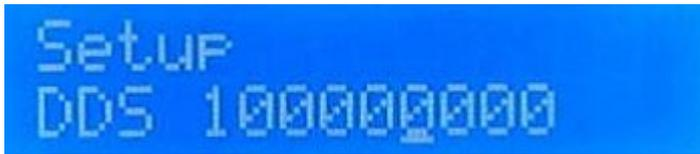
Set up the DDS clock. The default value is 125MHz. 100MHz is used in the kit. Press F+ and F- to set the above displayed value, 100000000. The cursor indicates the tuning rate. Press STEP to select 10Hz, 100Hz, 1KHz rate.
