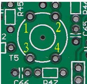
Install the MOSFETS. The leads of the MOSFET are labeled in the picture.
