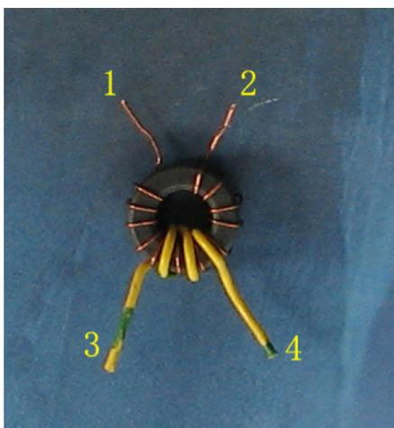
**T1** : Broadband transformer, 3-turn primary, 12-turn secondary, 0.31 enameled wire on FB-43-2402 core. The 3-turn primary is wound on middle part the secondary. For clearer instruction, the yellow wire is used as the primary. The photo shows the actual turns. Remove about 5 mm enamel from the leads, and tin. Cut 19.5 cm length of enameled wire for the 12-turn secondary, leaving about 1 cm for each lead. The length is the exact length for 12 turns with about 1 cm lead on each end. You wouldn't
