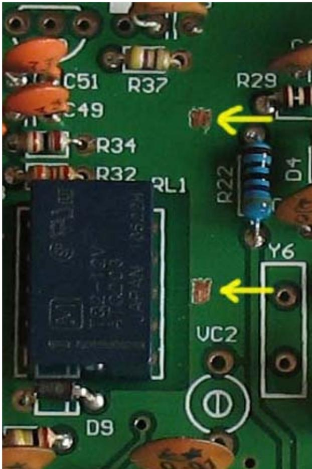
Remove a little green paint from the PCB in suitable position as indicated, and tin the two points.
