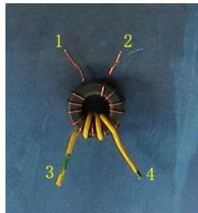
**T6, T7:** Broadband transformer, 5 bifilar turns 0.31 enameled wire on the binocular core made up of 2 small sleeves. Cut a pair of 12 cm long enameled wire, and thread through the core. Say Wire A is red, Wire B blue. Connect 2 (the finish of A) with 3 (the start of B) as the tap. You don't have to twist the wire. Leave about 1 cm for each lead. Remove about 5 mm enamel from the leads, and tin.
