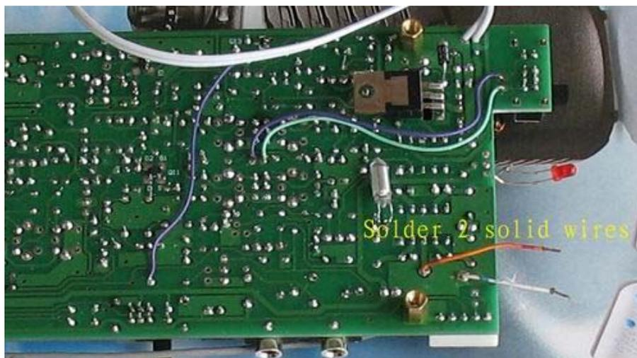
**Step 4:** Assemble the panel and solder the 2 wires to BNC. Fasten the 2 side screws.
