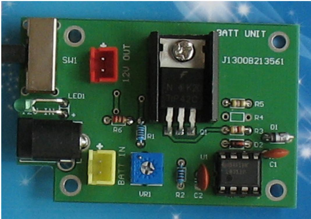
and height so that it aligns the indicator opening on the case side. Use the red connector for power output. Use the yellow connector for battery input. Q1 is hot at start of charging, so a heat sink is needed. R6 is the LED current limiting resistor. Value ranging from 1k – 5.6k is fine.
