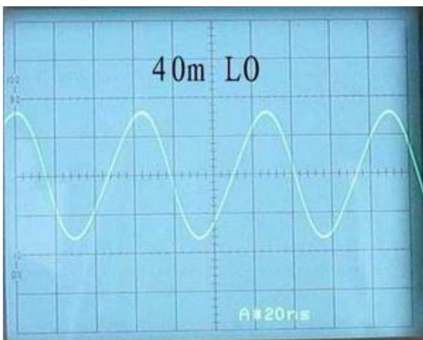
of L2 and C54. Turn TUNE to the reading is about 23.175MHz. Turn clockwise to the end. The reading is around 23.325MHz. Now, BAND 2 works from 14.175 - 14.325. Sacrificing the lower segment frequency would increase the upper frequency a few kilohertz. If you have an oscilloscope, remove the frequency counter and connect the probe to the joint of L2 and C54. Around 3 V p-p could be measured. The wave is perfect. Note: RL1 and D9 are
