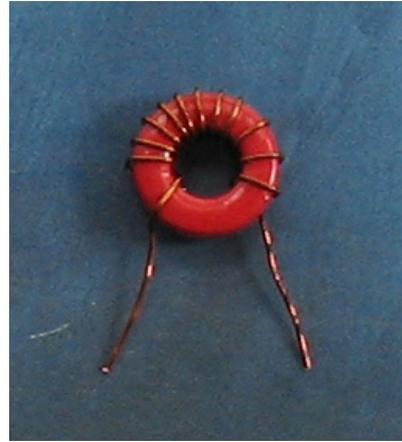
**L11, L12:** 20m LPF inductor, 12 t, 0.47 enameled wire on T37-2 core. Cut 16 cm long enameled wire. Leave about 1 cm for each lead. Remove about 5 mm enamel from the leads, and tin.
