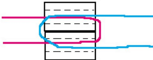
**T5:** Broadband transformer, 3-turn primary, 12-turn secondary, 0.31 enameled wire on FB-43-2402 core. The 3-turn primary is wound on middle part the secondary. Remove about 5 mm enamel from the leads, and tin.
