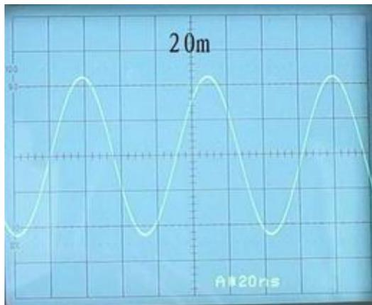
Switch MODE to CW. Short-circuit KEY, 4W could be measured. If you have an oscilloscope, connect the probe to the dummy load. 40V p-p could be measured at the dummy load. Trim L5 and L6 to peak. Switch MODE to LSB. Talk to MIC, 40V p-p could be measured.
