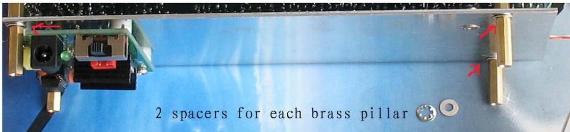
Place two spring washers to raise the height of the 4 pillars to 17 mm. If four thicker spring washers are supplied, place one washer for each pillar.
