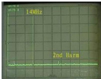
TJ2A complies with the FCC spectral purity requirement. The output spurious signals are 43dB below the carrier.
