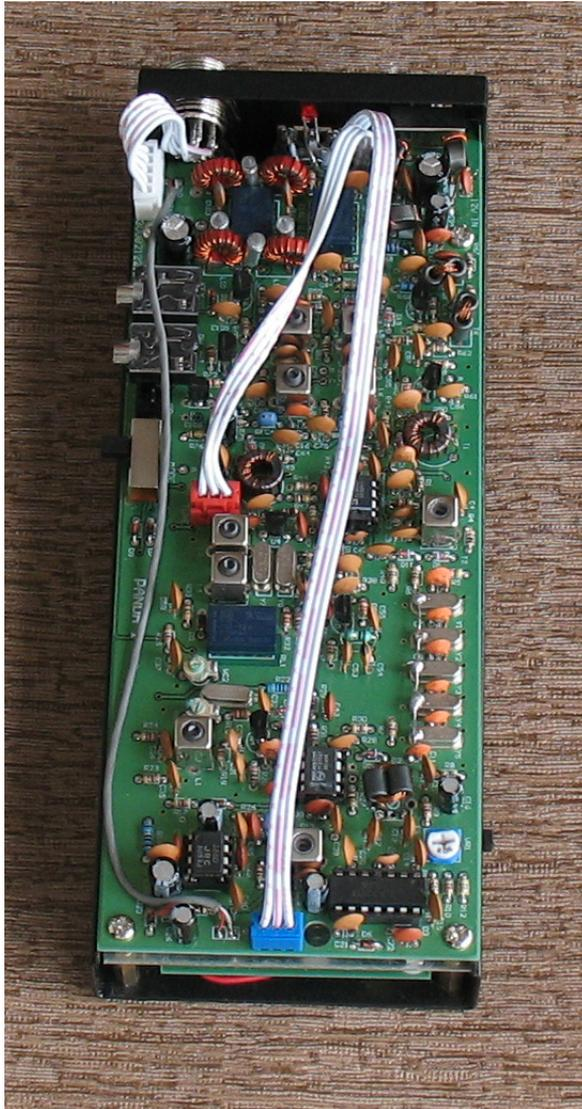
Before the top cover is placed, it is suggested to test the rig again. Receiving works? Transmission works? Calibrate the frequency. Everything is fine. Then we close the top cover.
