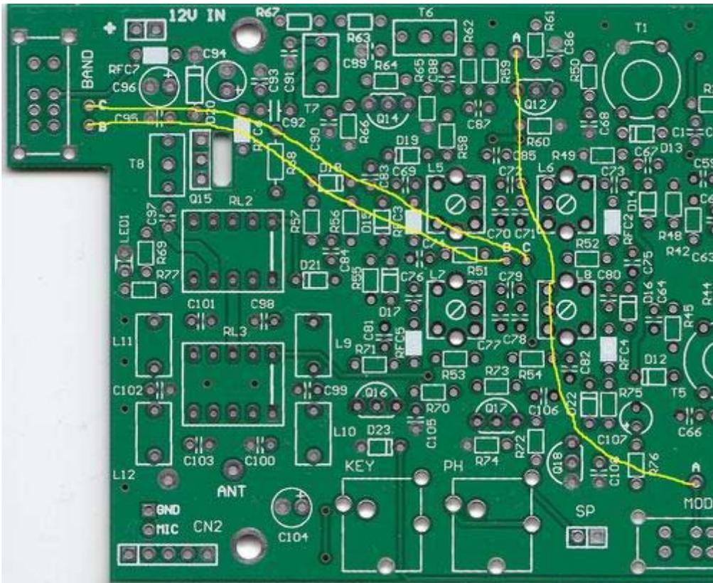
Connect the pots of TUNE and AF GAIN. The GND arm of the pot (labeled GND in the picture) should be connected to the square pad. Otherwise the tuning or the AF GAIN direction would be reversed. Never short-circuit the right side arm of TUNE pot to the ground. This would damage U4.
