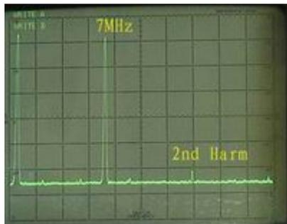
470 ohm, even 220 should be used for R62 to reduce the gain. How to determine R62 then? Use 680 ohm for R62 (Don't cut the resistor too short. Leave about 5 mm leads). Set MODE to LSB. Press PTT, but do not talk to MIC. If power appears, R62 should be reduced. You don't have to remove the resistor. Simply parallel a 1K resistor to R62. Press PTT again. If power still appears, remove the 1K, resistor and parallel a 470 ohm to R62. Now, the problem usually is solved.
