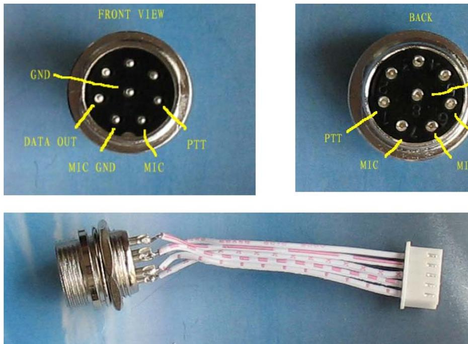
Solder the aviation plug pins to the 5-line cord according to the definition. It is suggested the cord be kept as short as possible (the original length is fine). Plug this 5-pin connector to CN2 of the main board. Do not run the 5-line cable too close to L10 and L12. Keep the cable to the case side.
