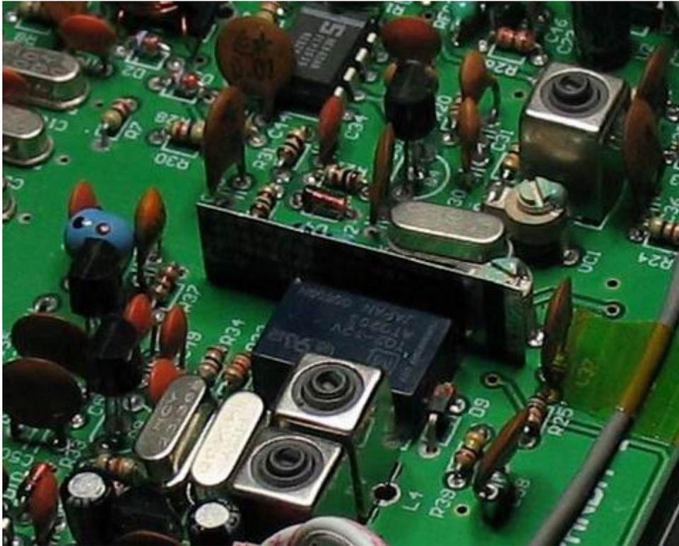
Place the metal strip in such a place as to separate VC2 from RL1.
