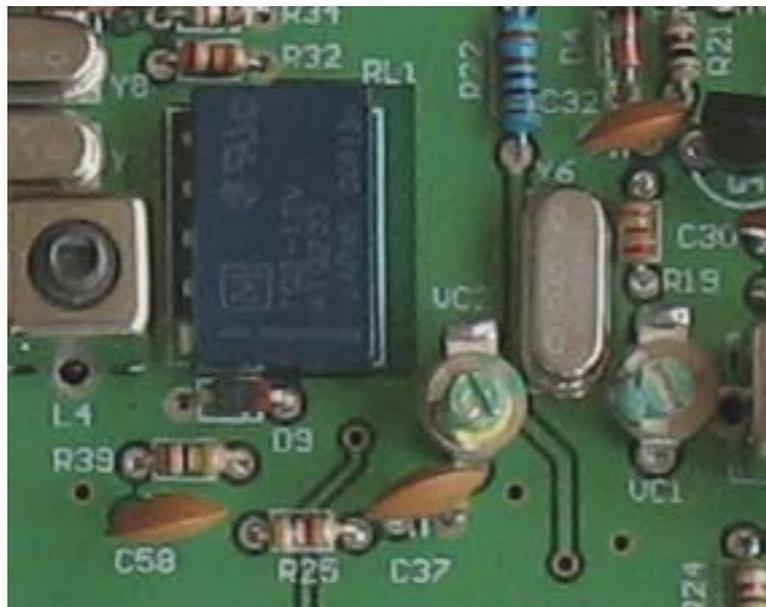
and the PCB. Do not cut the diode leads short. Bend the leads to suit the pads and solder.
