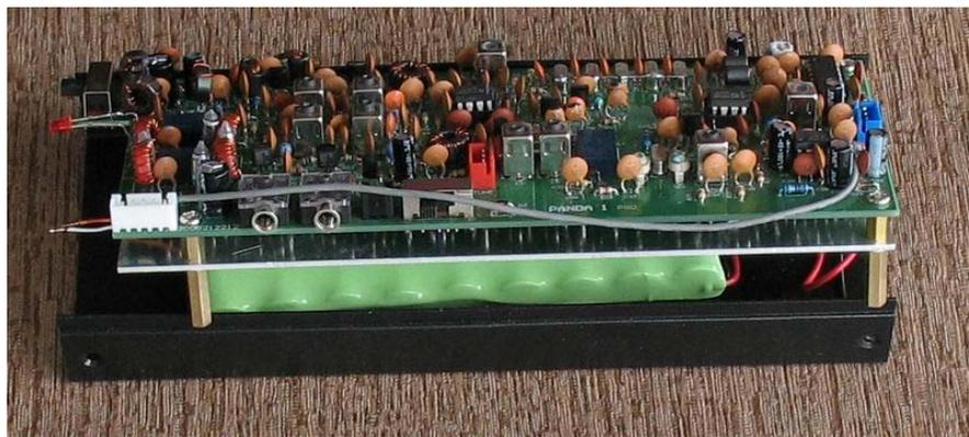
**Step 3:** Solid wires to the ANT pads. A length of 4 cm solid wire will do. Keep the 2 wires as short as possible. The GND wire is shorter.
