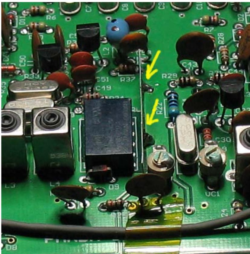
Cut a piece of metal strip measuring 28 × 10mm (this could be obtained from the canned food casing). Place it between RL1 and VC2. Do not place the metal strip too close against RL1 or VC1. Place it along the copper line beside RL1 (i.e., to leave some clearance from either RL1 or VC1) and solder (see picture below). You have to remove a little green
