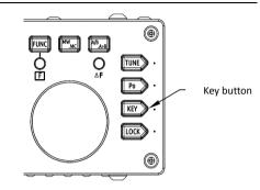
The [KEY] button function contains adjustment items that are commonly used when doing CW communication:
