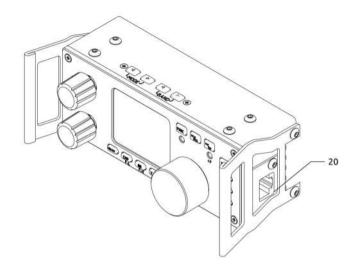
**20 MIC Interface** (On the right side of the machine-head) Connecting the multi-function MIC to this connector.
