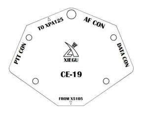
PTT CON PTT signal / BAND signal output port. The PTT signal of this port is completely isolated from the host,
